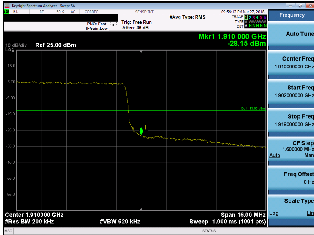
Plot 7-262. Upper Band Edge Plot (Band 2 - 20.0MHz QPSK - Full RB Configuration)
