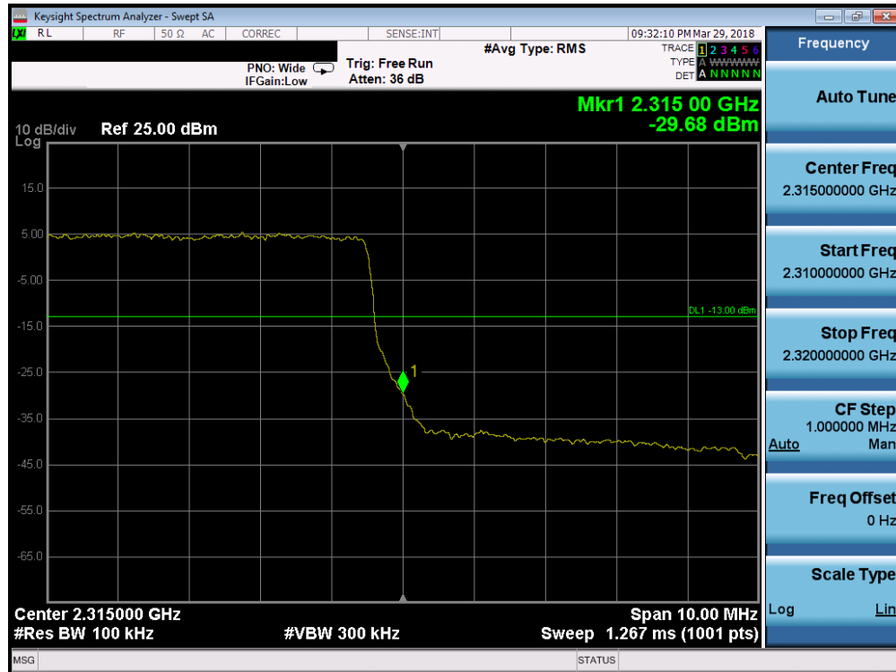
Plot 7-272. Upper Band Edge Plot (Band 30 - 10.0MHz QPSK - Full RB Configuration)
