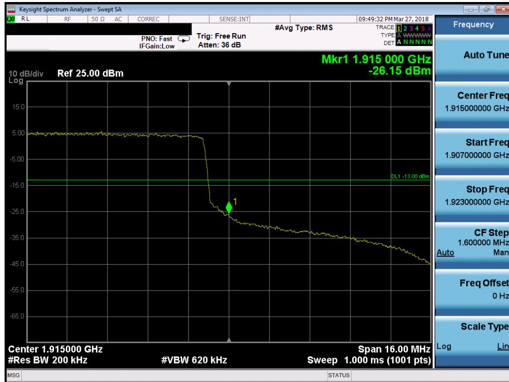
Plot 7-264. Upper Band Edge Plot (Band 25 - 20.0MHz QPSK - Full RB Configuration)
