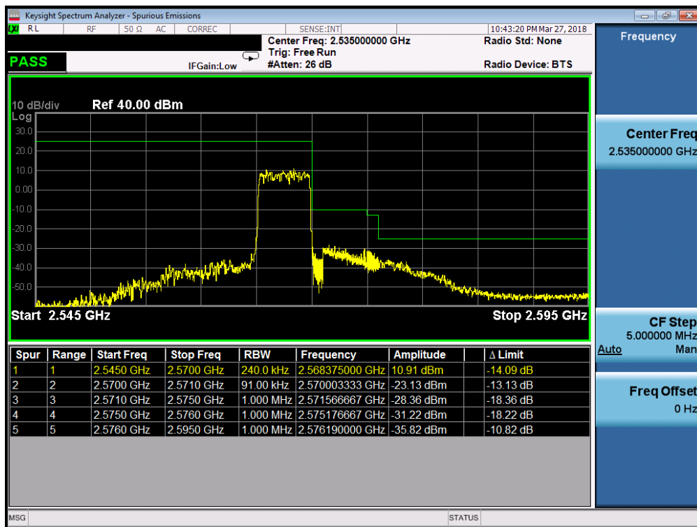
Plot 7-4. Upper ACP Plot (Band 7 – 5.0MHz QPSK – RB Size 25)
