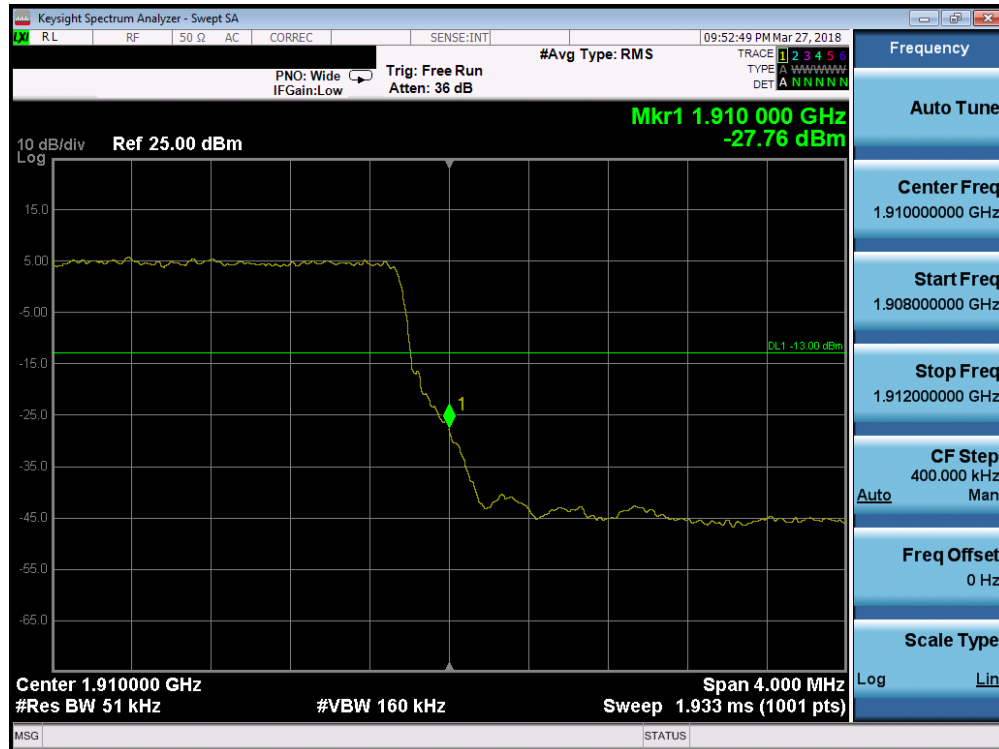
Plot 7-244. Upper Band Edge Plot (Band 2 - 5.0MHz QPSK - Full RB Configuration)
