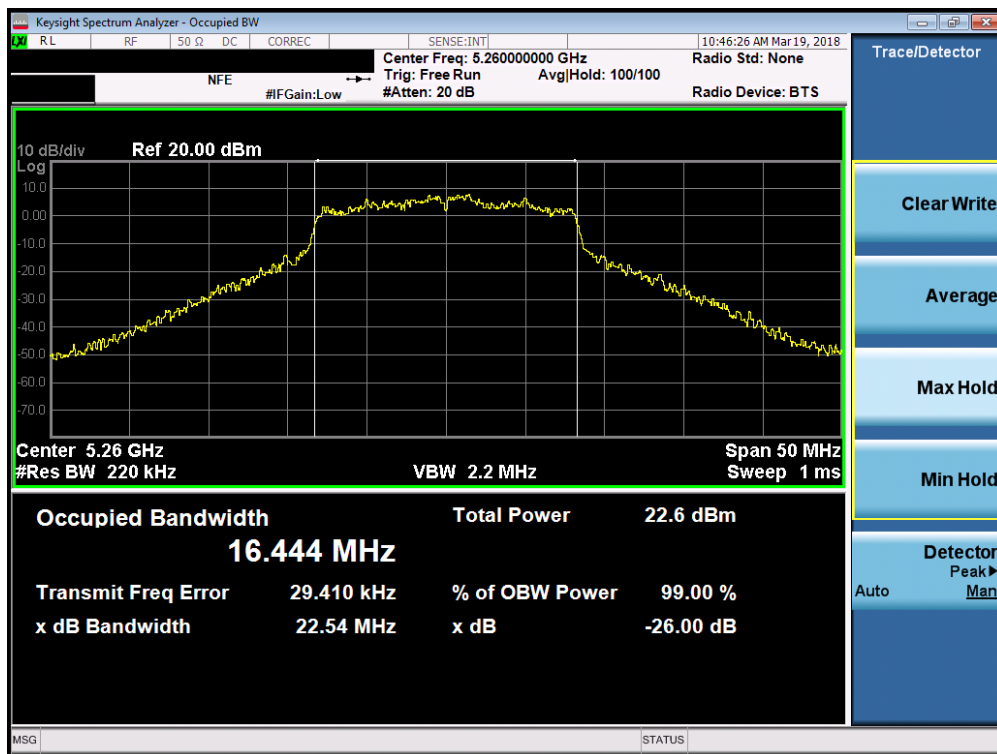
Plot 7-10. 26dB Bandwidth Plot SISO ANT1 (802.11a (UNII Band 2A) – Ch. 52)
