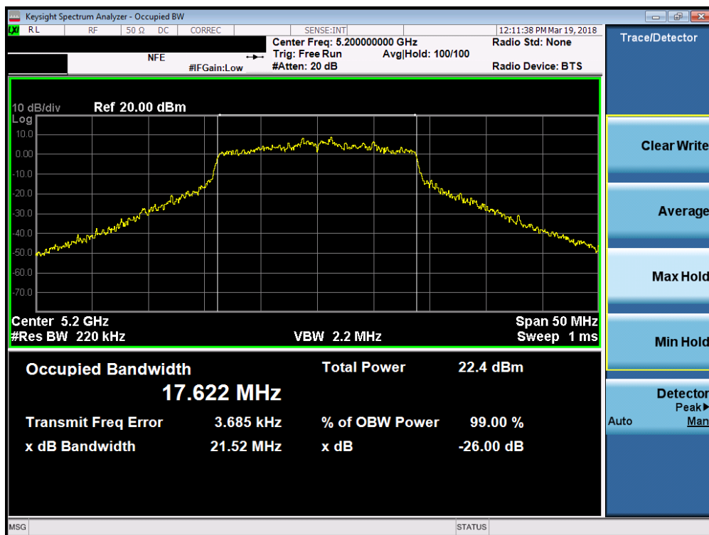
Plot 7-5. 26dB Bandwidth Plot SISO ANT1 (20MHz BW 802.11n (UNII Band 1) – Ch. 40)
