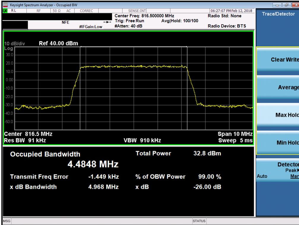
Plot 7-8. Occupied Bandwidth Plot (5MHz QPSK – RB Size 25– Low Channel)
