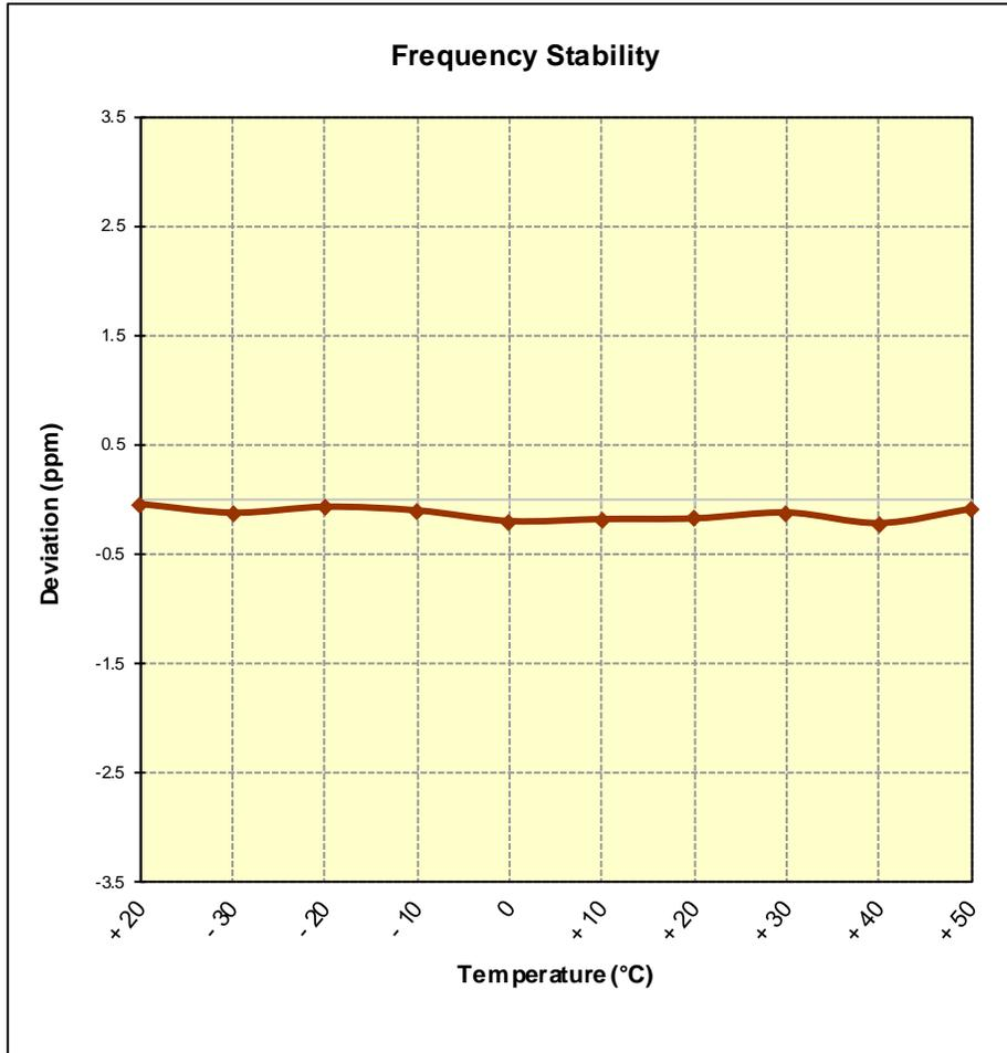
**Figure 7-6. CDMA BC10 Frequency Stability Graph (Ch. 670)**
