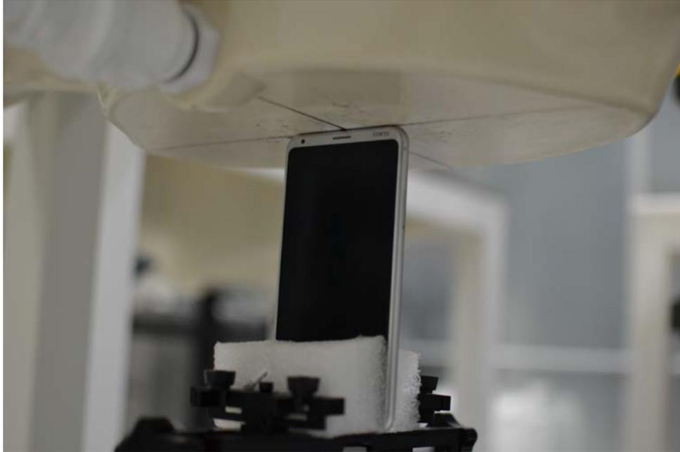
**SAR Test Setup Photo 11: Top at 0.0 cm**
