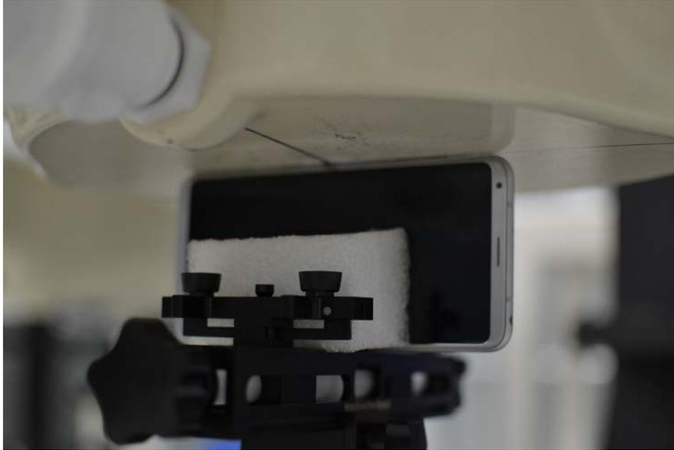
SAR Test Setup Photo 15: Left at 0.0 cm
