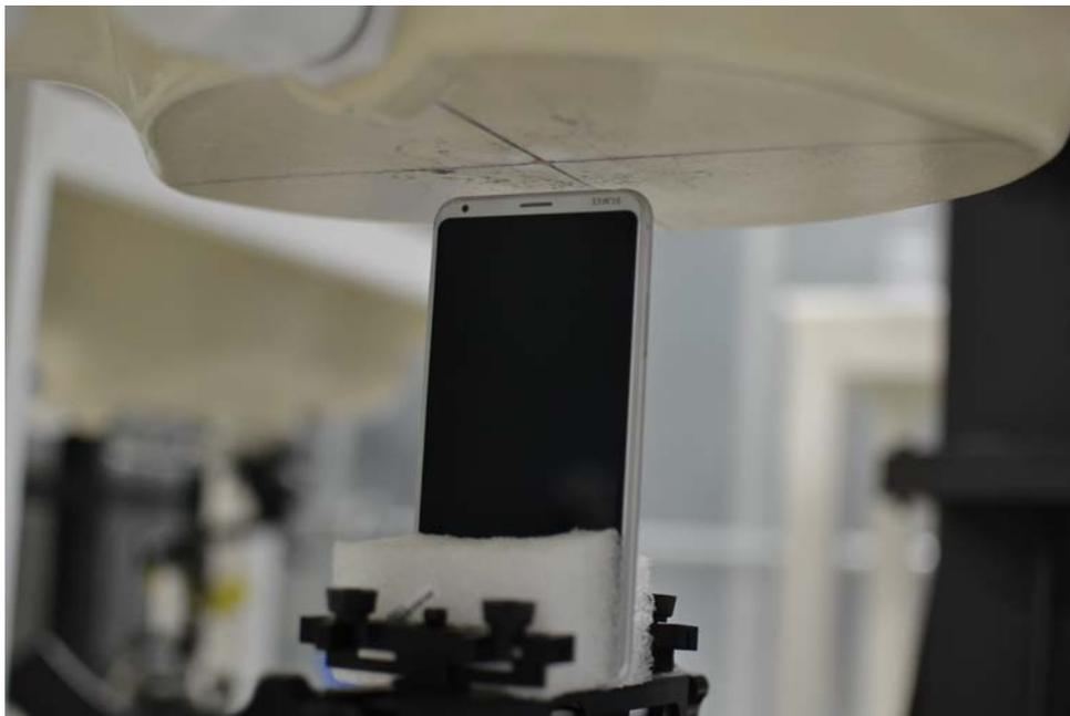
SAR Test Setup Photo 10: Top at 1.0 cm
