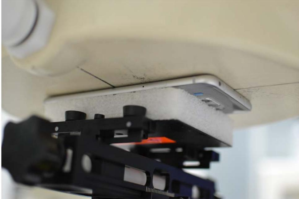
SAR Test Setup Photo 9: Front at 0.0 cm
