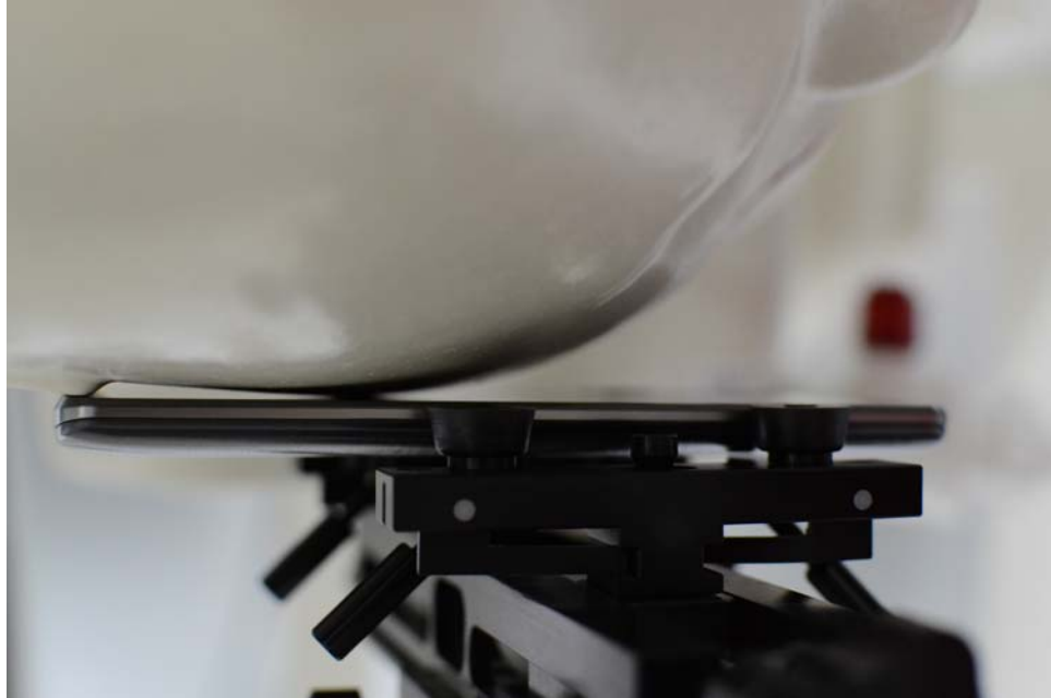
SAR Test Setup Photo 1: Right Cheek
