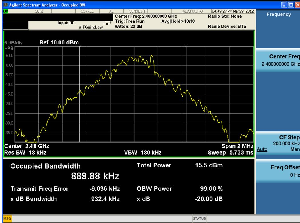
Plot 6-3. 20dB Bandwidth Plot (Bluetooth, 1Mbps – Ch. 78)
