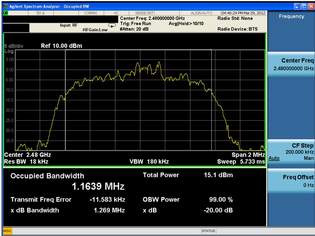
Plot 6-9. 20dB Bandwidth Plot (Bluetooth, 3Mbps – Ch. 78)
