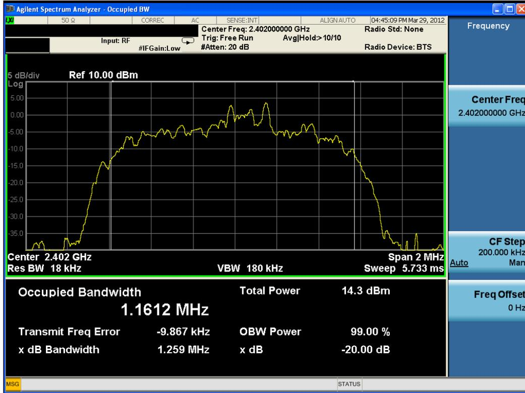
Plot 6-7. 20dB Bandwidth Plot (Bluetooth, 3Mbps – Ch. 0)
