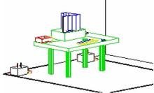
**Figure 3-3. Wooden Table & Bonded LISNs**
