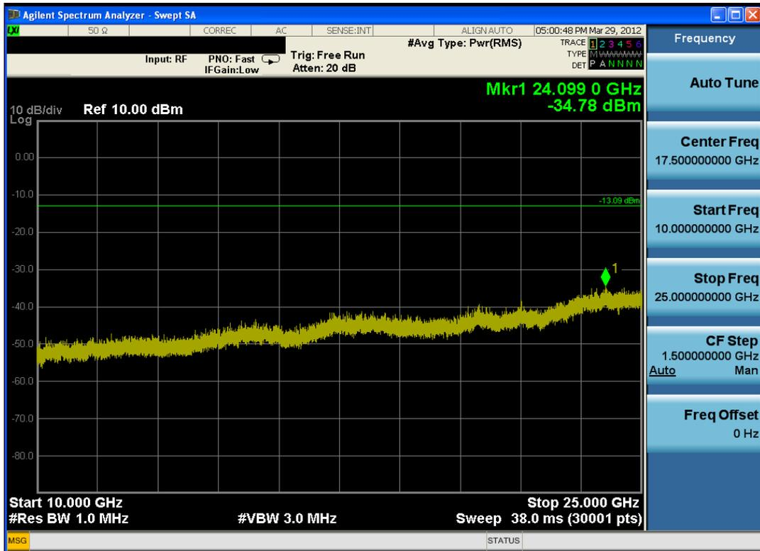
Plot 6-23. Conducted Spurious Plot (Bluetooth, 3Mbps – Ch. 78)
