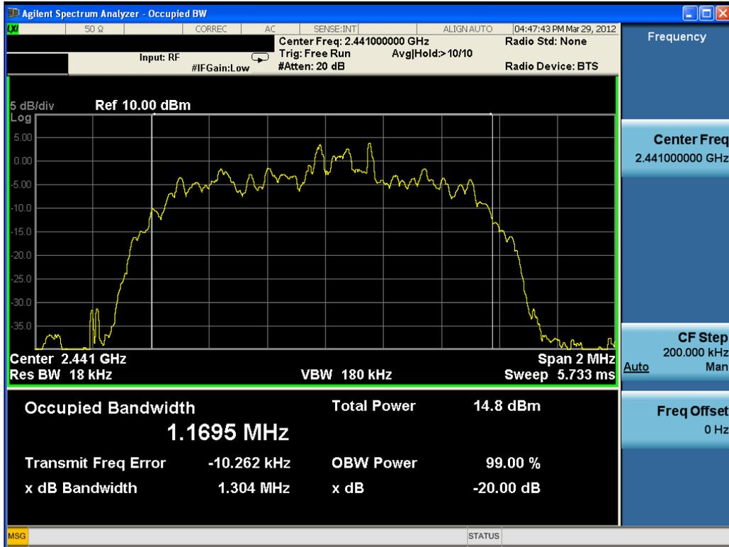
Plot 6-5. 20dB Bandwidth Plot (Bluetooth, 2Mbps – Ch. 39)
