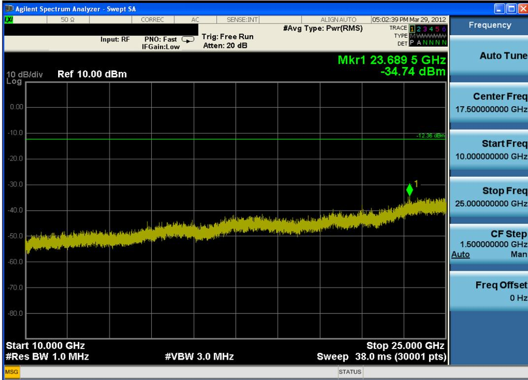
Plot 6-21. Conducted Spurious Plot (Bluetooth, 3Mbps – Ch. 39)
