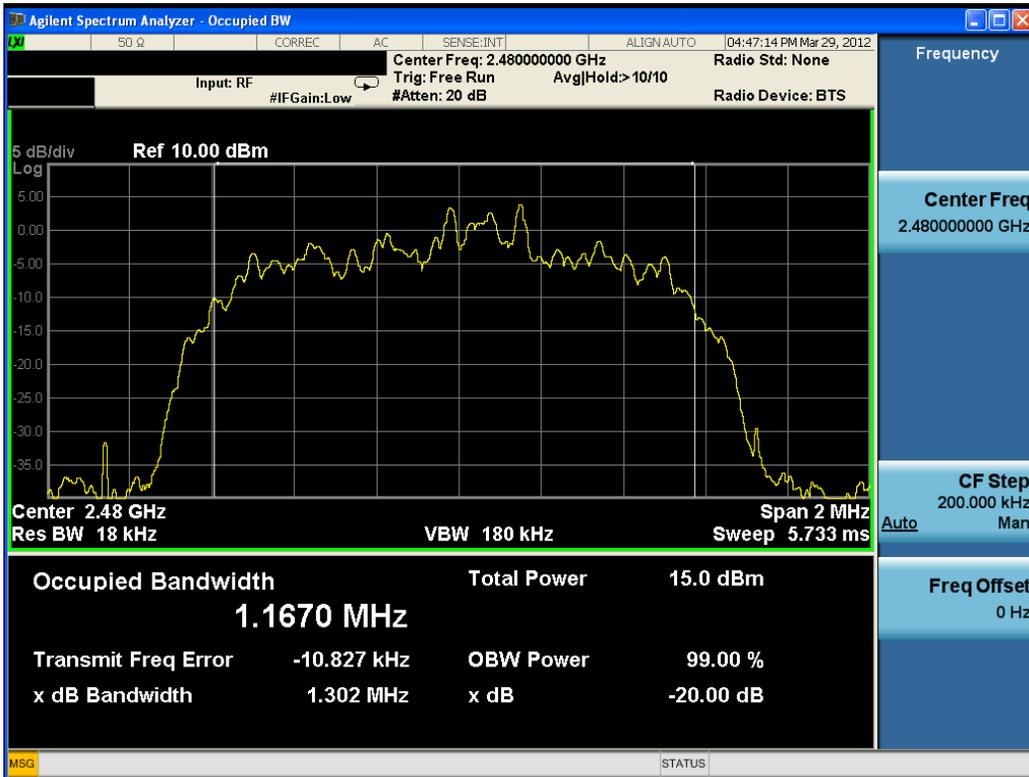
Plot 6-6. 20dB Bandwidth Plot (Bluetooth, 2Mbps – Ch. 78)
