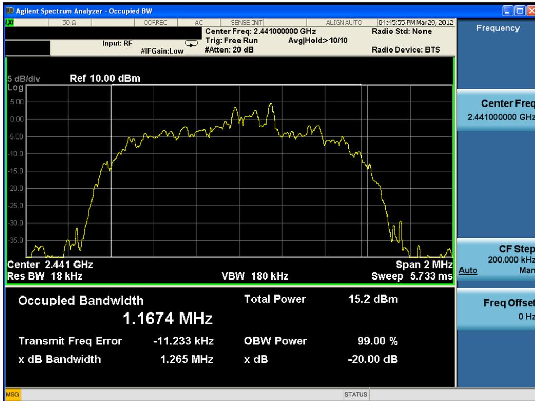
Plot 6-8. 20dB Bandwidth Plot (Bluetooth, 3Mbps – Ch. 39)
