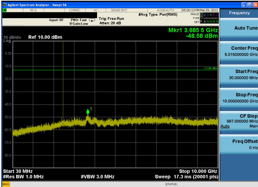
Plot 6-22. Conducted Spurious Plot (Bluetooth, 3Mbps – Ch. 78)
