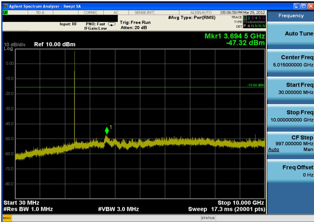
Plot 6-18. Conducted Spurious Plot (Bluetooth, 3Mbps – Ch. 0)
