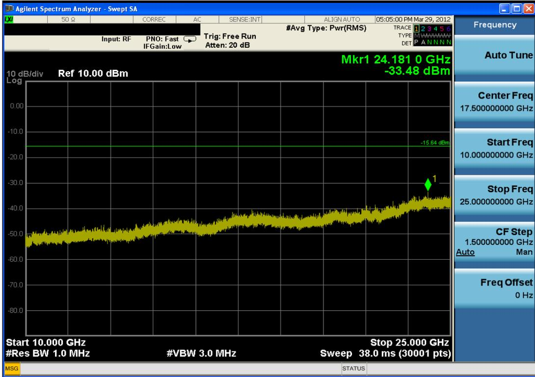
Plot 6-19. Conducted Spurious Plot (Bluetooth, 3Mbps – Ch. 0)
