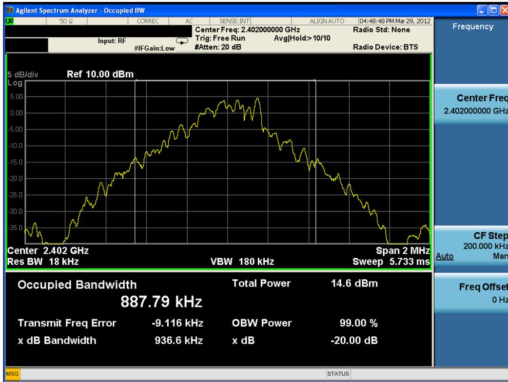
Plot 6-1. 20dB Bandwidth Plot (Bluetooth, 1Mbps – Ch. 0)
