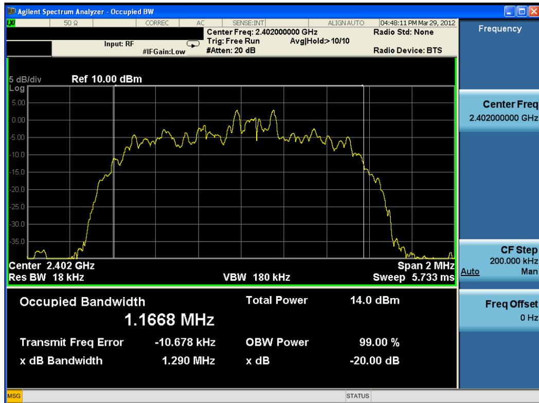
Plot 6-4. 20dB Bandwidth Plot (Bluetooth, 2Mbps – Ch. 0)
