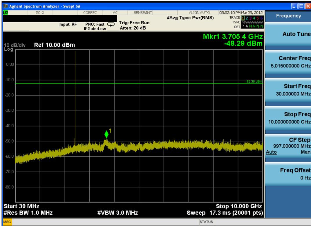
Plot 6-20. Conducted Spurious Plot (Bluetooth, 3Mbps – Ch. 39)
