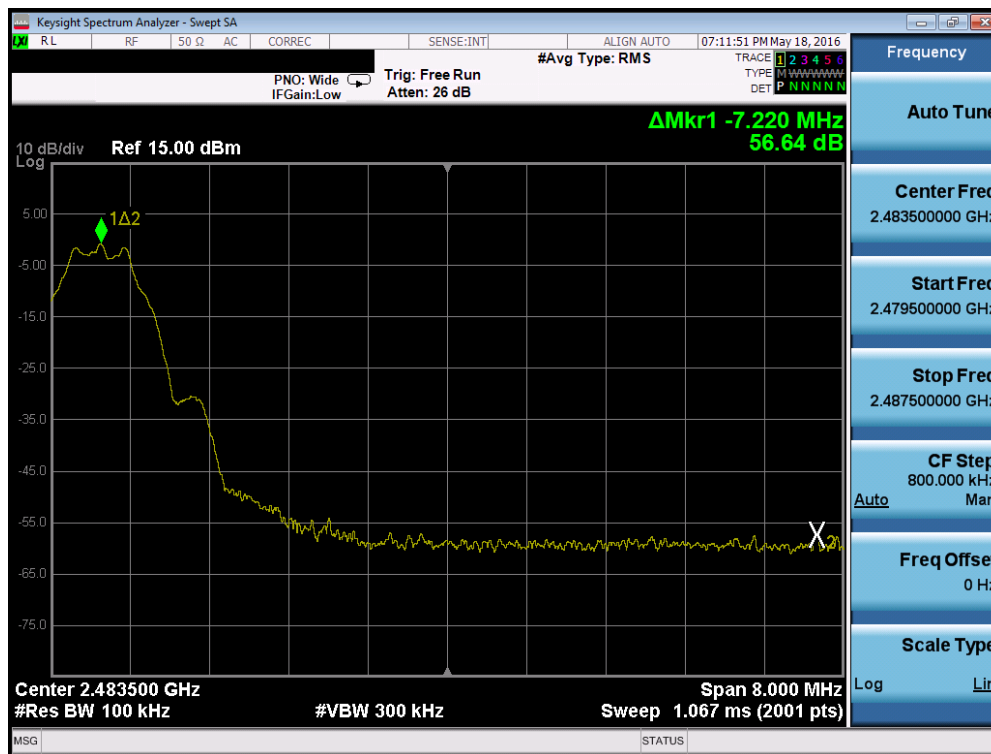
Plot 7-11. Band Edge Plot (Bluetooth (LE) – Ch. 39)
