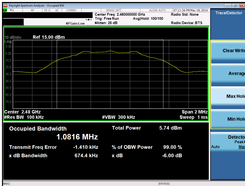
Plot 7-3. 6dB Bandwidth Plot (Bluetooth (LE) – Ch. 39)
