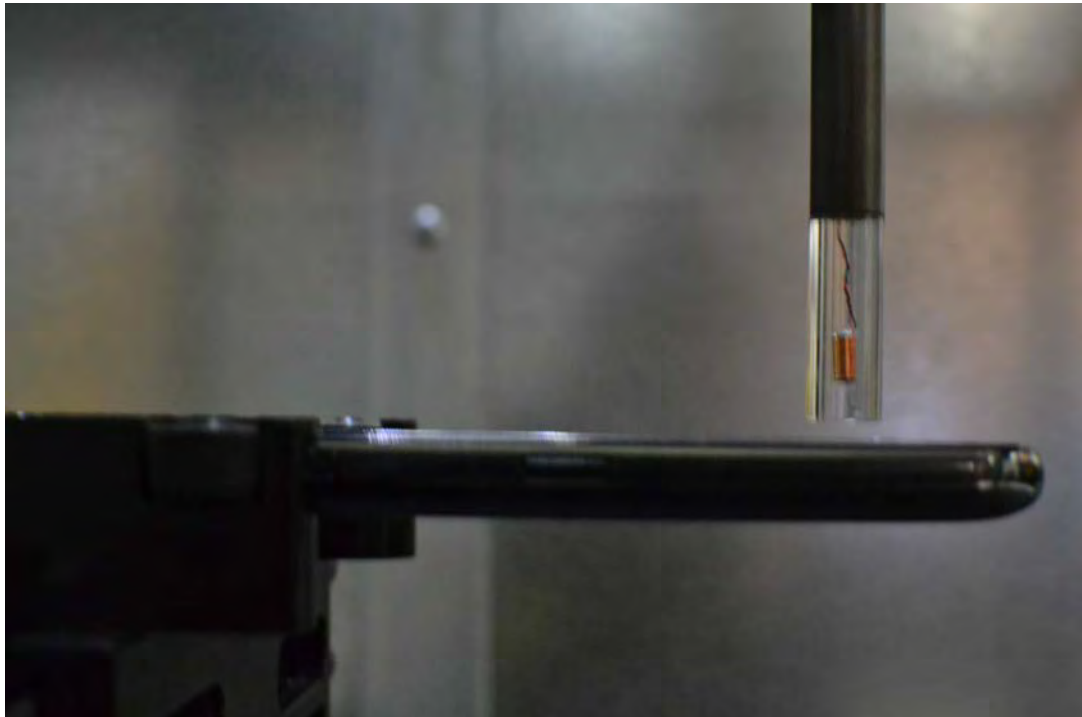
Figure 13-2 Test Setup for Wireless Device
