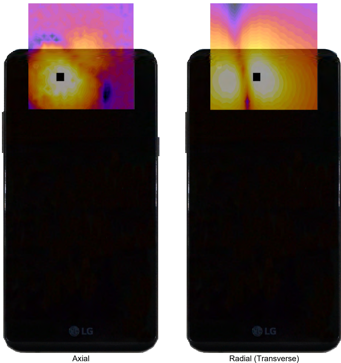
Figure 13-3 T-Coil Scan Overlay Magnetic Field Distributions
