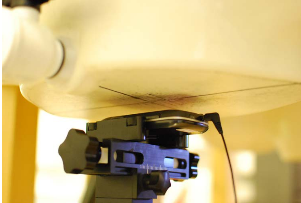
SAR Test Setup Photo 5 – Body-worn at 1.5 cm
