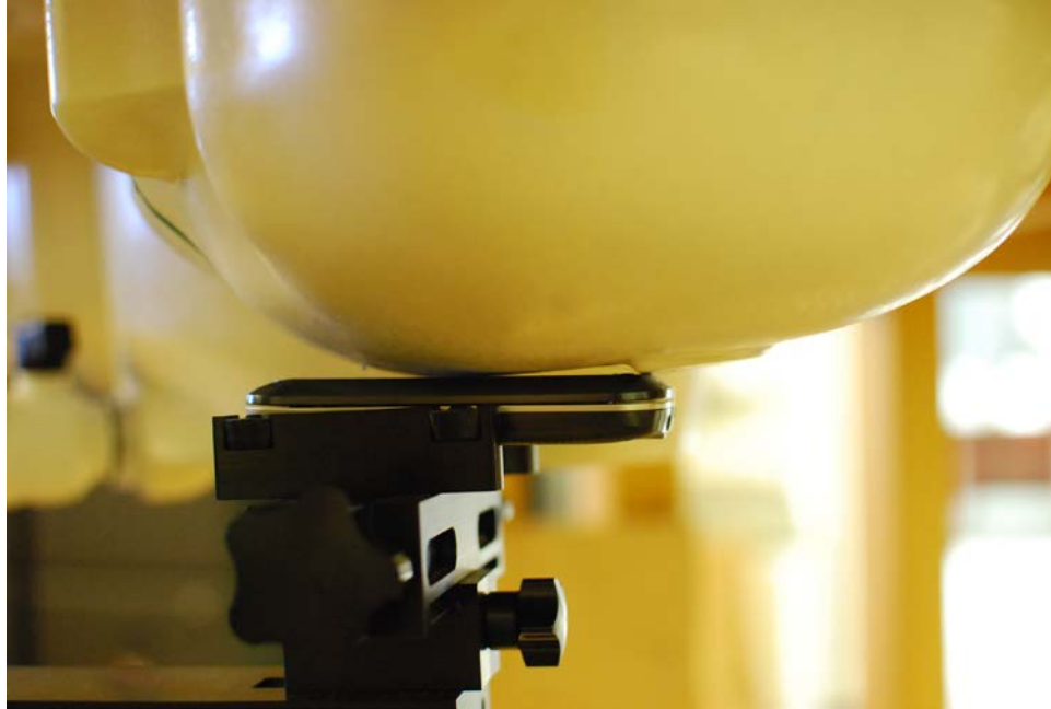
SAR Test Setup Photo 3 – Left Touch
