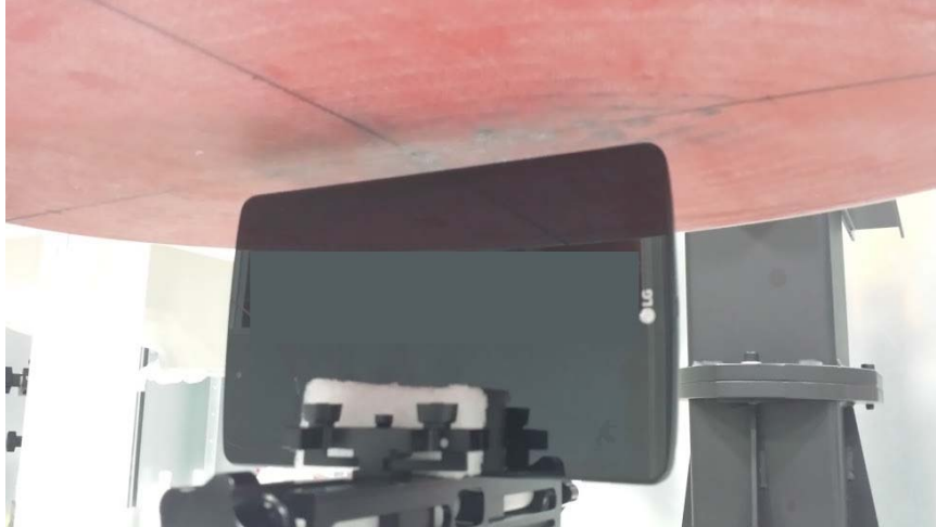
SAR Test Setup Photo 5: Right Edge at 0.7 cm
