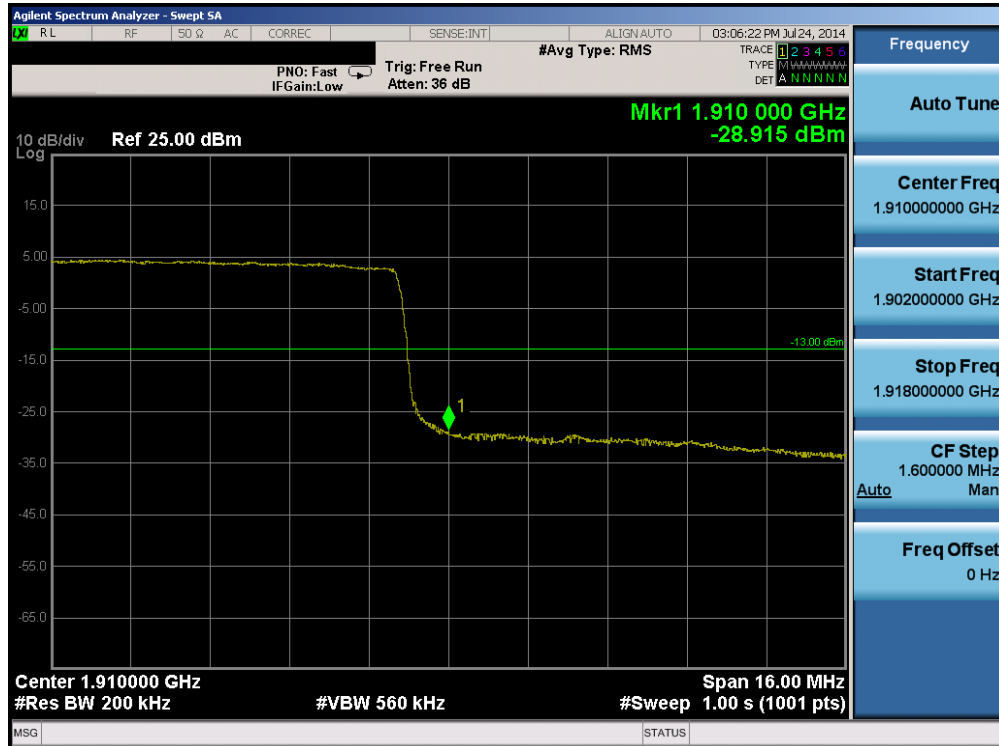
Plot 6-93. Upper Band Edge Plot (Band 2 – 20.0MHz QPSK – RB Size 100)
