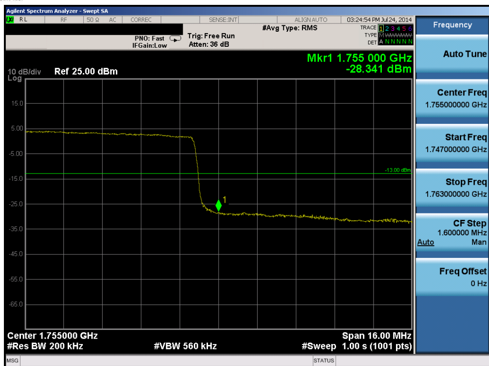
Plot 6-77. Upper Band Edge Plot (Band 4 – 20.0MHz QPSK – RB Size 100)
