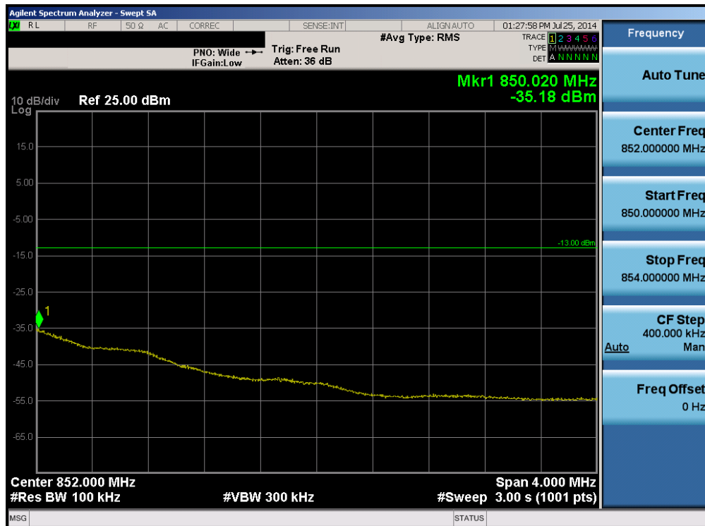
Plot 6-52. Upper Extended Band Edge Plot (Band 5 – 1.4MHz QPSK – RB Size 6)
