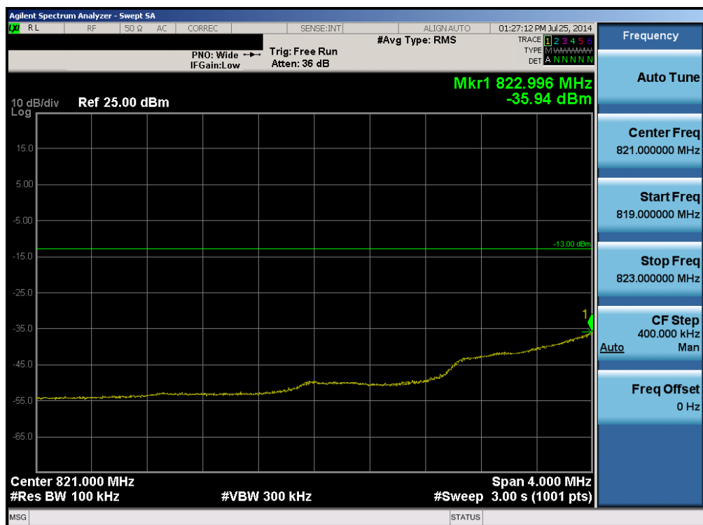
Plot 6-50. Lower Extended Band Edge Plot (Band 5 – 1.4MHz QPSK – RB Size 6)
