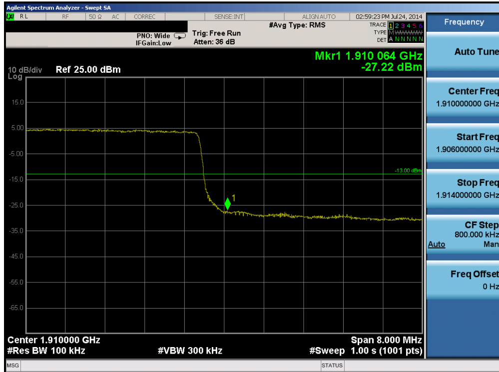
Plot 6-85. Upper Band Edge Plot (Band 2 – 10.0MHz QPSK – RB Size 50)
