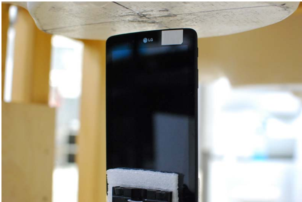
SAR Test Setup Photo 4 – Top Edge at 16 mm
