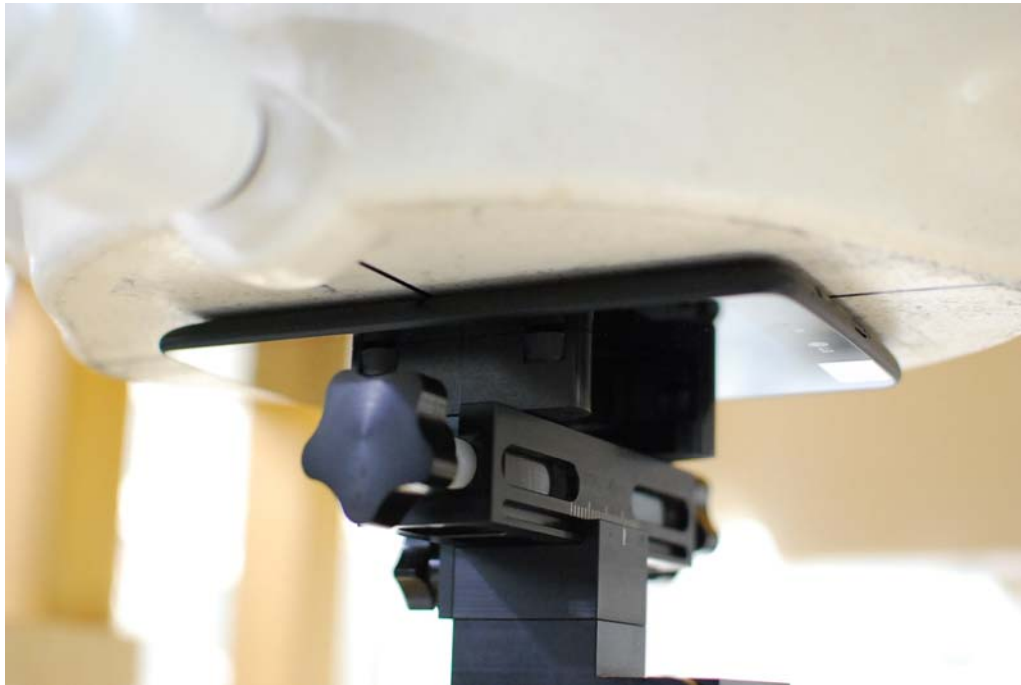
SAR Test Setup Photo 1 – Back Side at 0.0 mm
