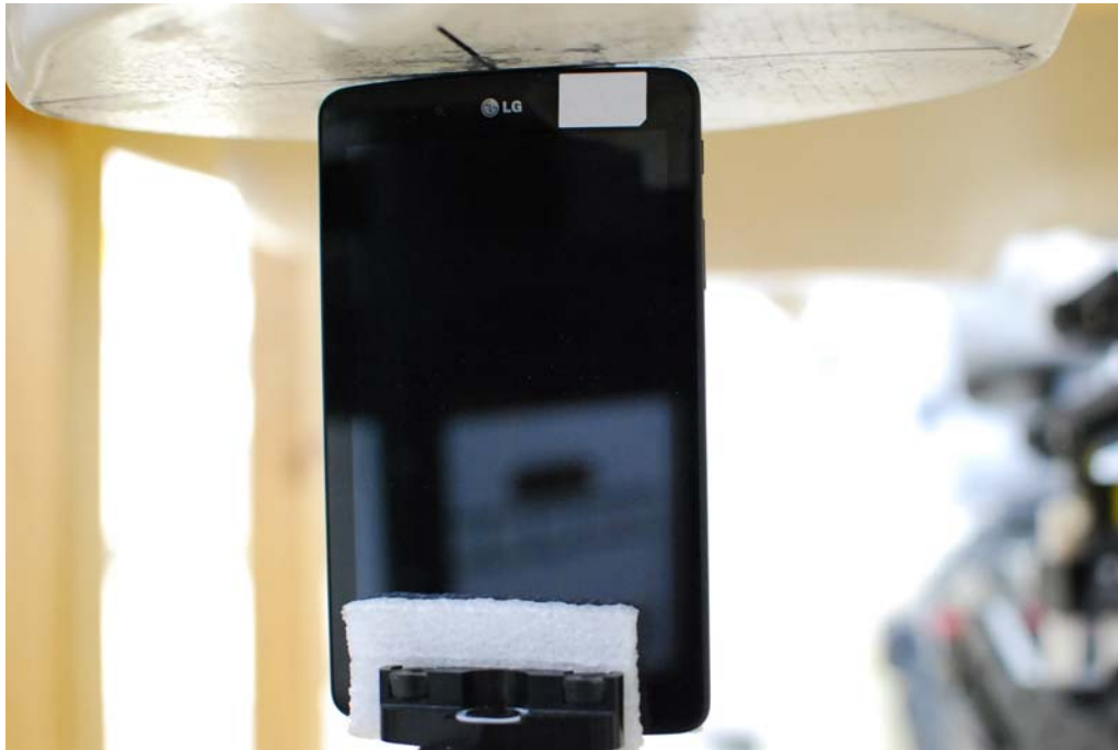
SAR Test Setup Photo 3 – Top Edge at 0.0 mm
