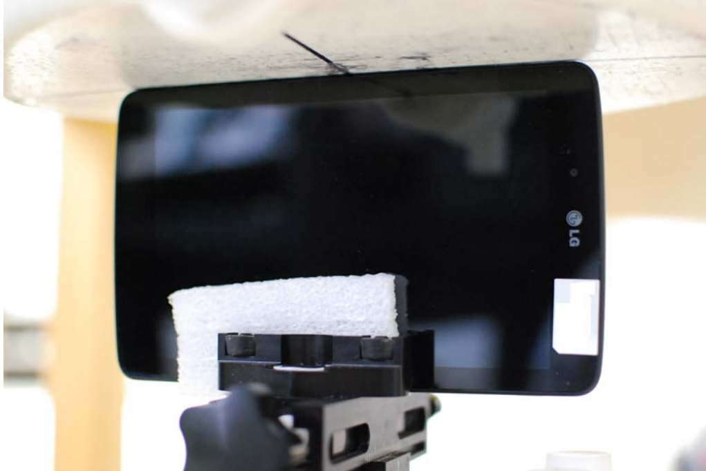
SAR Test Setup Photo 7 – Left Edge at 0.0 mm
