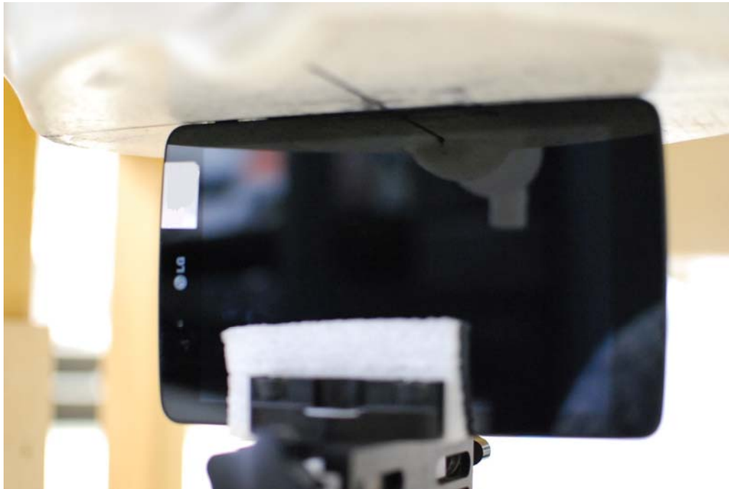
SAR Test Setup Photo 5 – Right Edge at 0.0 mm
