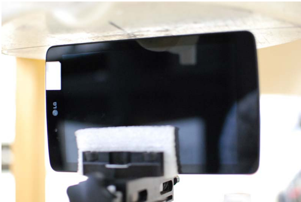
SAR Test Setup Photo 6 – Right Edge at 5.0 mm
