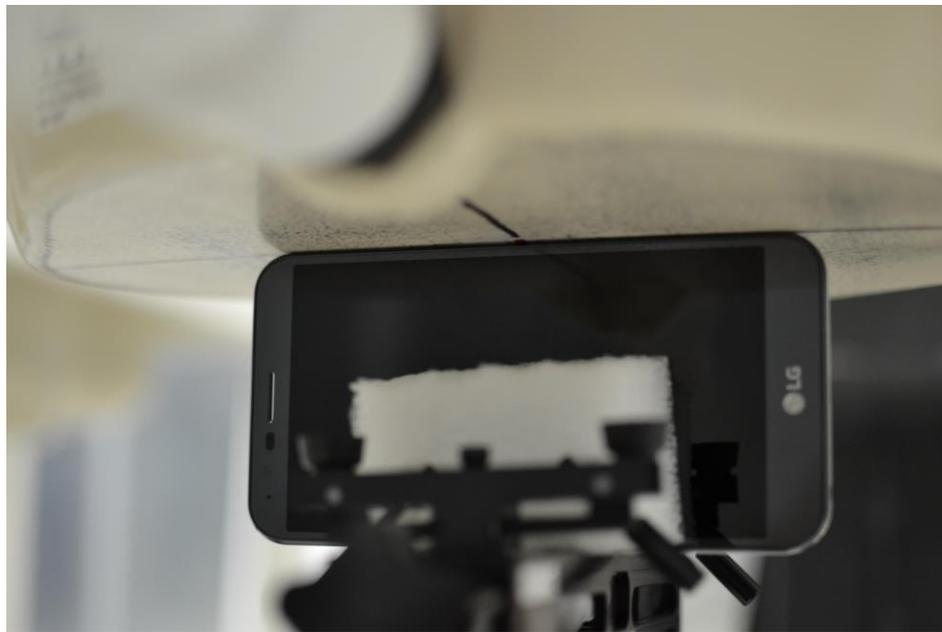
SAR Test Setup Photo 14 – Right at 0.0 cm
