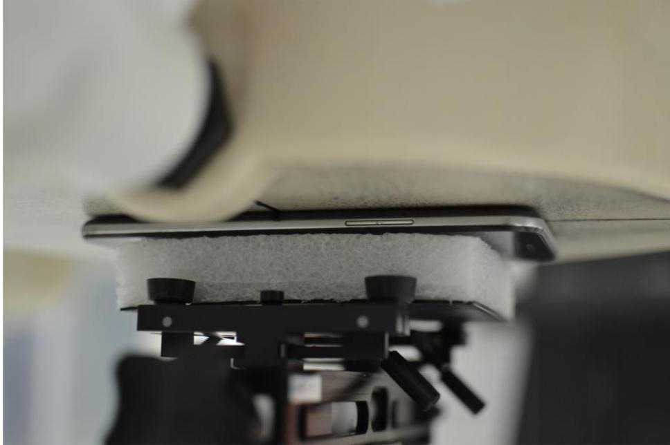
SAR Test Setup Photo 11 – Back at 0.0 cm
