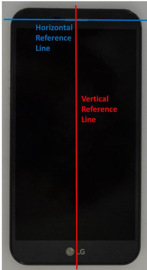
**SAR Test Setup Photo 14 – Vertical and Horizontal Reference Lines**
