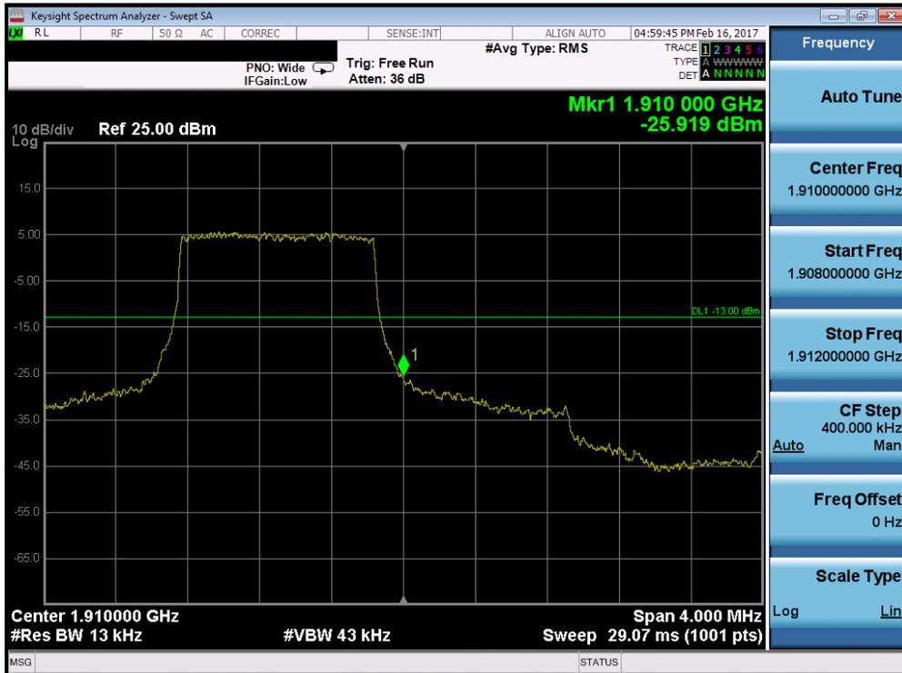
Plot 7-160. Upper Band Edge Plot (Band 2 – 1.4MHz QPSK – RB Size 6)
