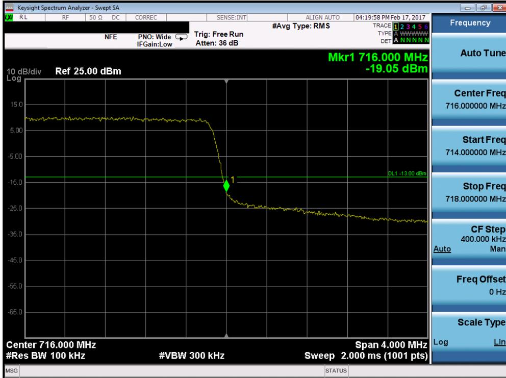
Plot 7-121. Upper Band Edge Plot (Band 12 – 3.0MHz QPSK – RB Size 15)
