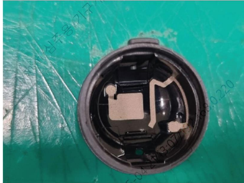
Figure E-2 Antenna Location (Bottom Side View)
