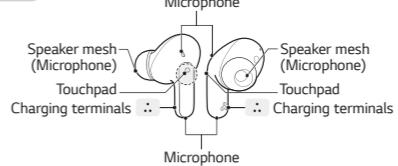
\*Make sure that the charging terminal is not soiled with foreign substance.
