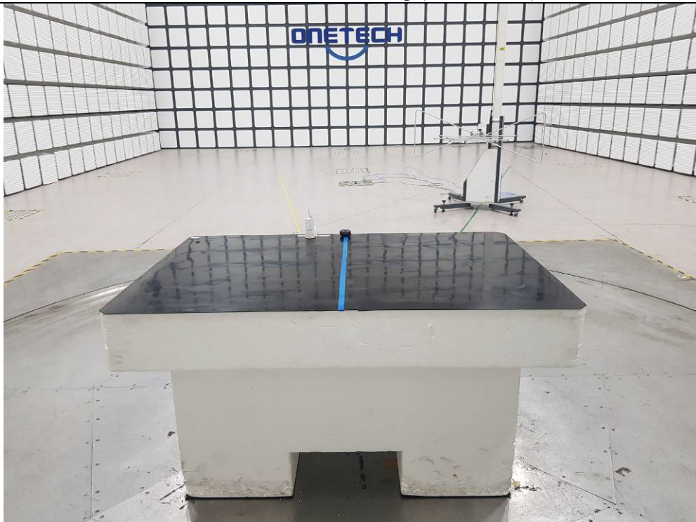
Radiated Emission Test Set Up (Below 1 GHz)
