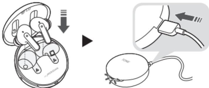
When the charging cable is connected, the charging status is displayed in the charging case.
