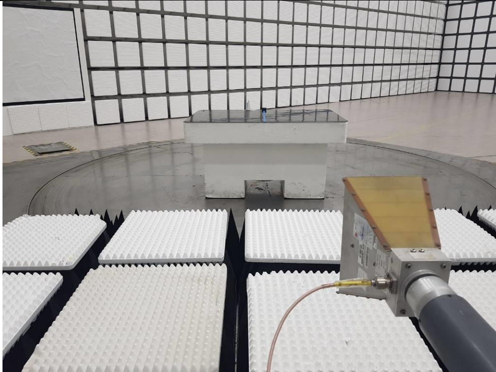
Radiated Emission Test Set Up (Above 1 GHz)
