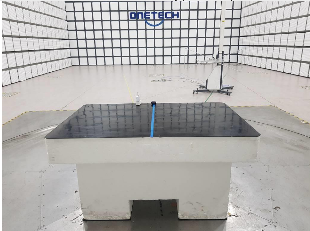
Radiated Emission Test Set Up (Below 1 GHz)
