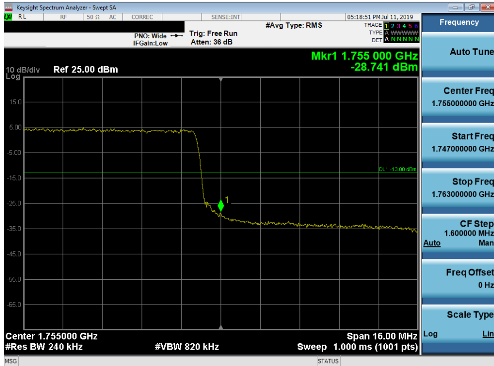
Plot 7-244. Upper Band Edge Plot (Band 4 - 20.0MHz QPSK - Full RB Configuration)
