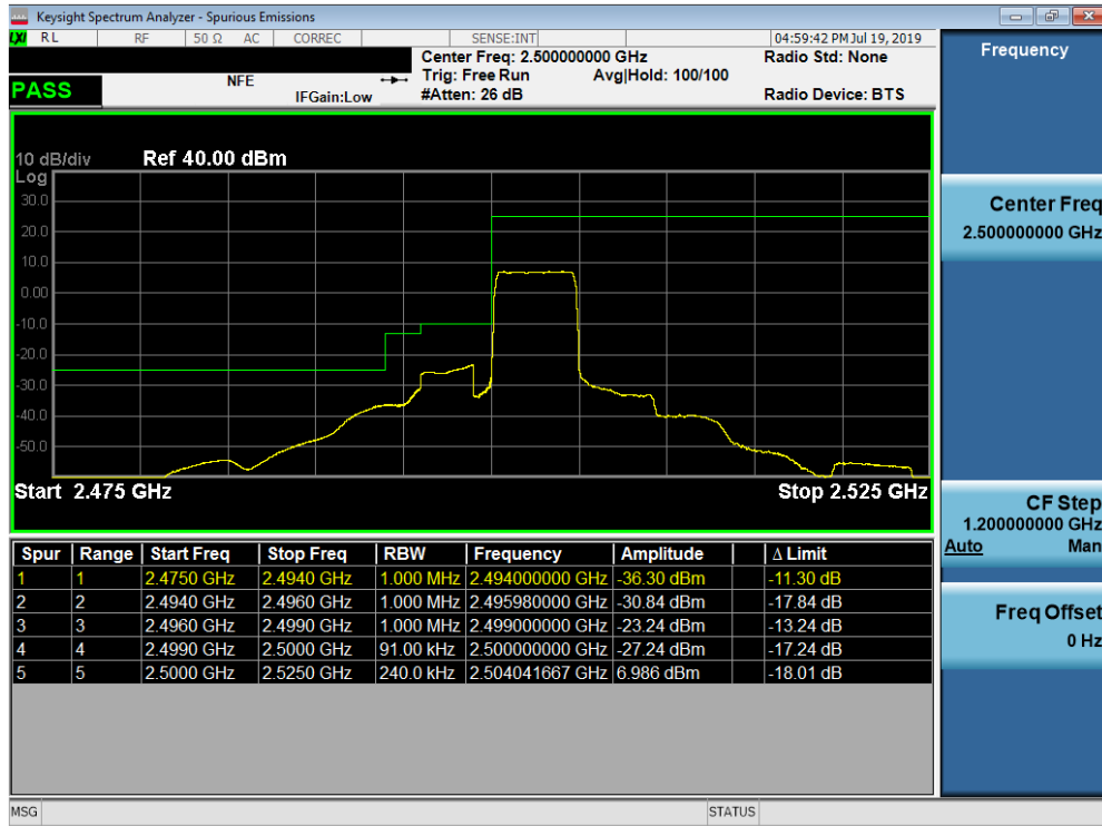
Plot 7-284. Lower ACP Plot (Band 7 - 5.0MHz QPSK - Full RB Configuration)
