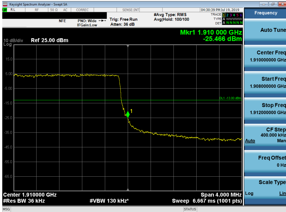
Plot 7-256. Upper Band Edge Plot (Band 2 - 3.0MHz QPSK - Full RB Configuration)
