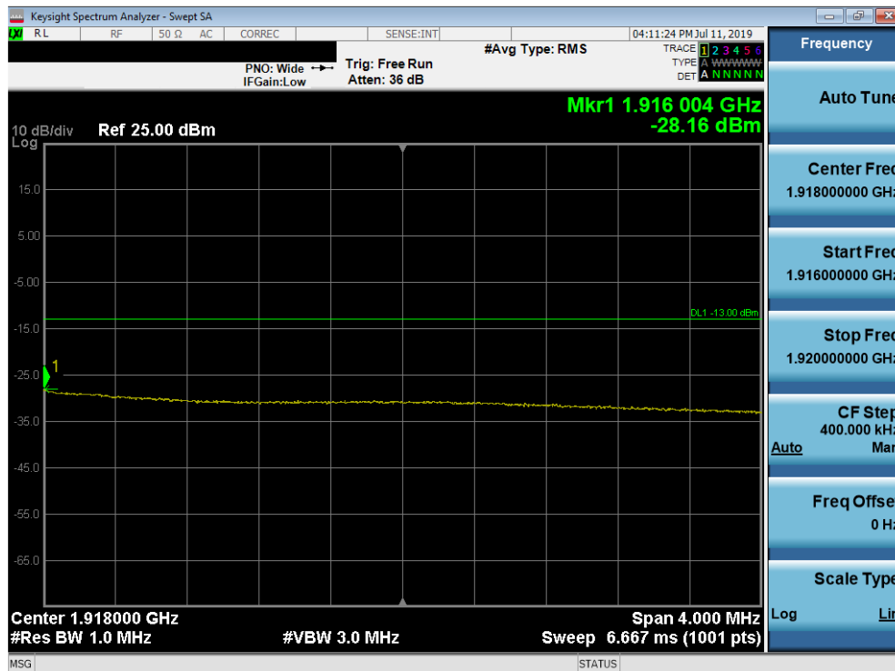
Plot 7-277. Upper Extended Band Edge Plot (Band 25 - 15.0MHz QPSK - Full RB Configuration)
