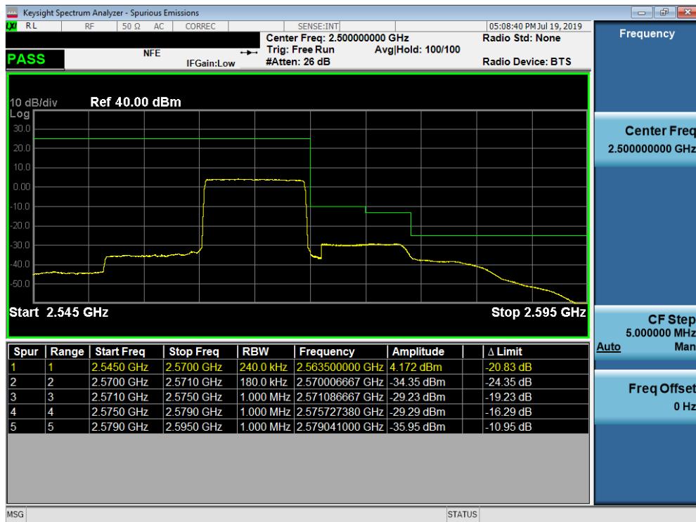
Plot 7-287. Upper ACP Plot (Band 7 - 10.0MHz QPSK - Full RB Configuration)
