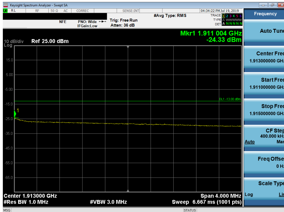
Plot 7-269. Upper Extended Band Edge Plot (Band 2 - 10.0MHz QPSK - Full RB Configuration)
