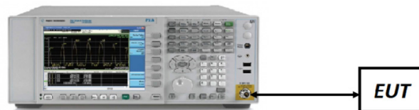
Figure 7-2. Test Instrument & Measurement Setup
