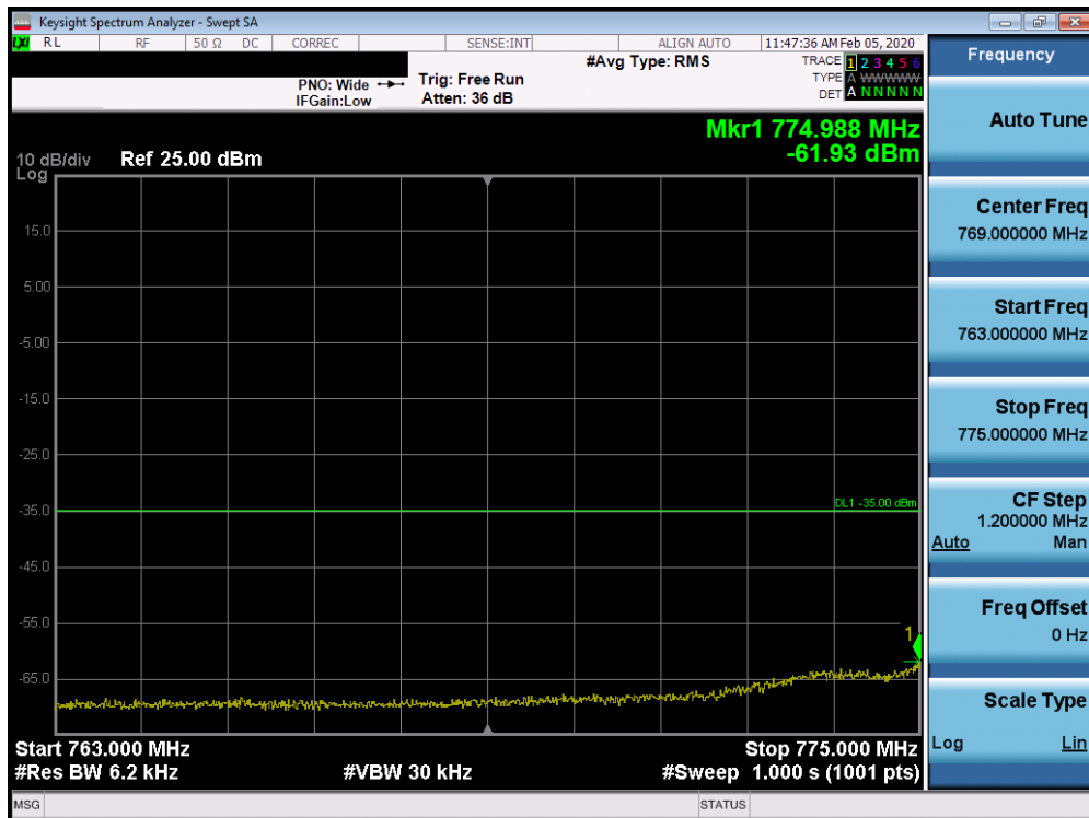
Plot 7-172. Lower Emission Mask Plot (Band 13 - 10.0MHz QPSK - Full RB Configuration)
