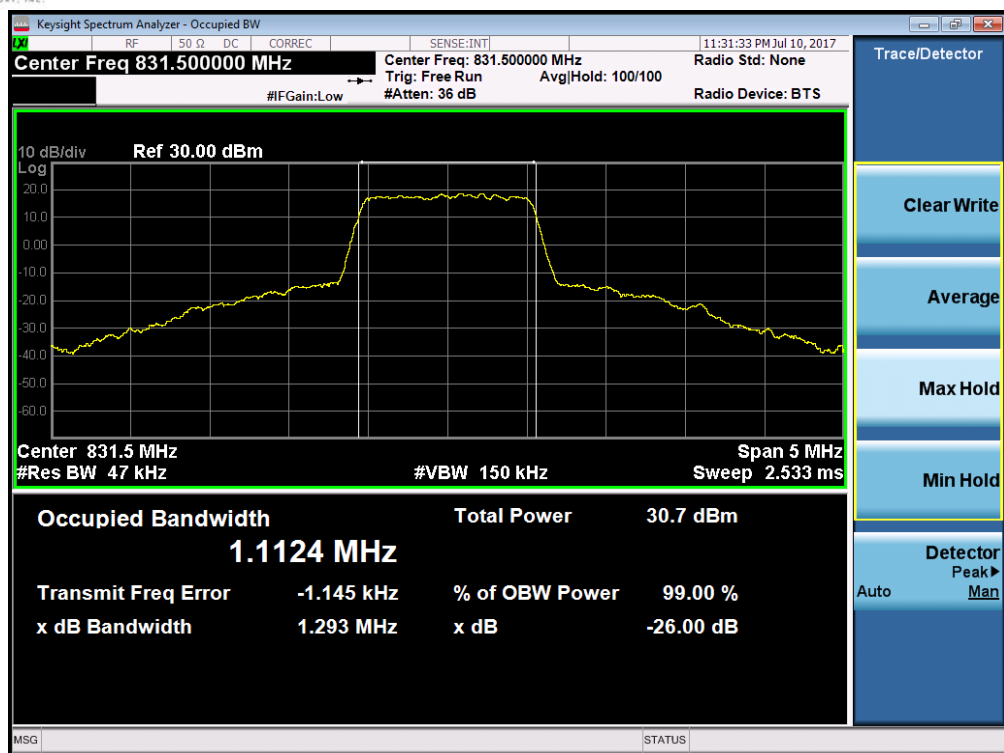
Plot 7-13. Occupied Bandwidth Plot (Band 26/5 – 1.4MHz QPSK – RB Size 6)
