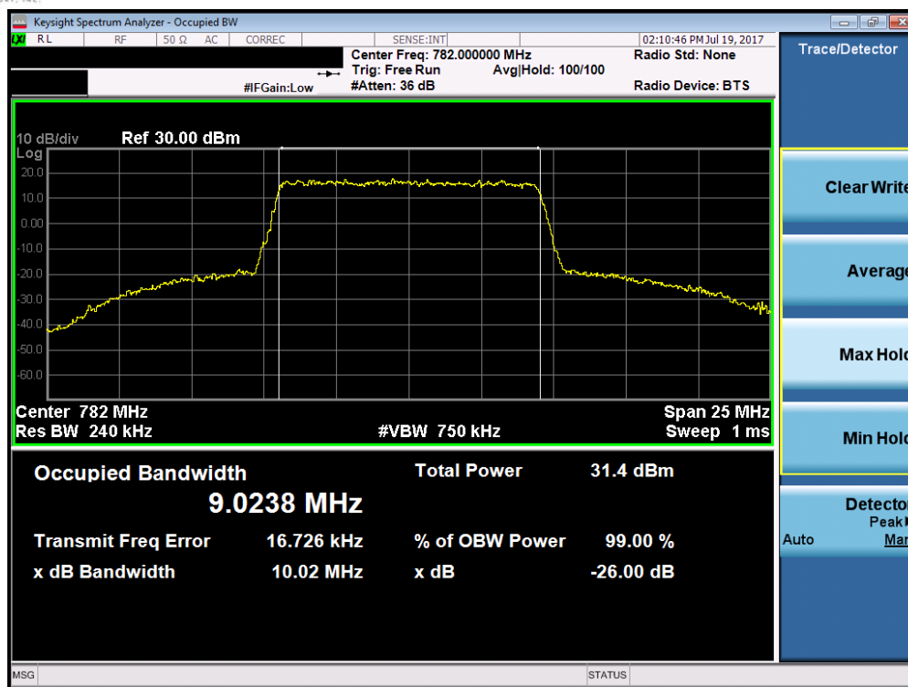
Plot 7-11. Occupied Bandwidth Plot (Band 13 – 10.0MHz QPSK – RB Size 50)
