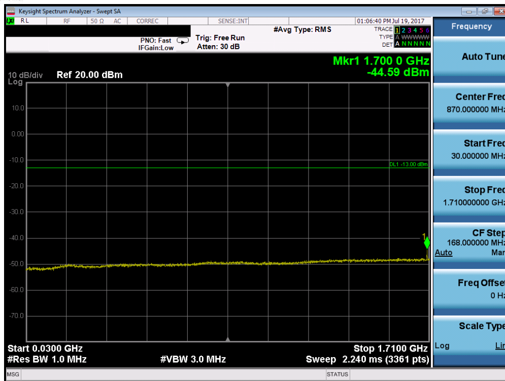
Plot 7-85. Conducted Spurious Plot (Band 4 – 15.0MHz QPSK – RB Size 1, RB Offset 0 – Mid Channel)
