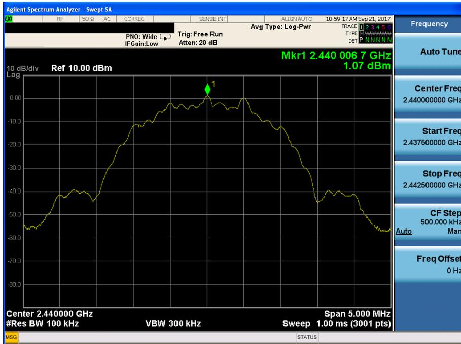
TM 2 Conducted Spurious Emissions 1 (Test Channel : Middle)
