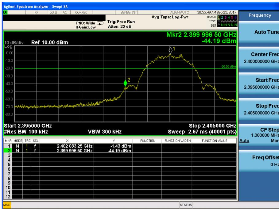
TM 2 Conducted Spurious Emissions 1 (Test Channel : Lowest)
