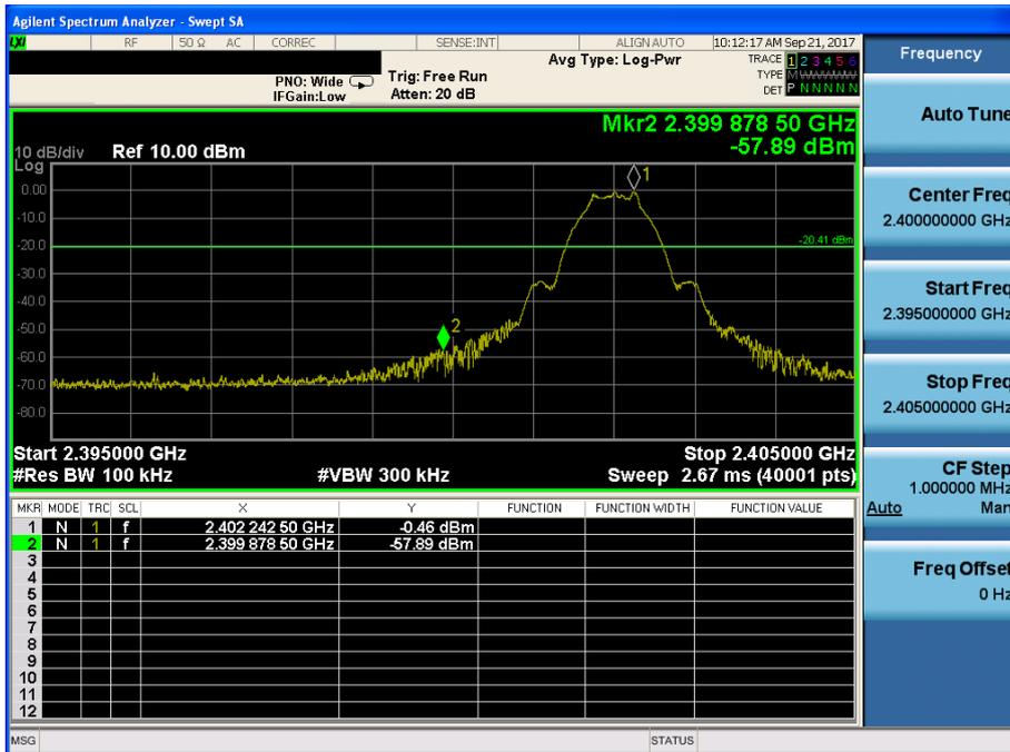
TM 1 Conducted Spurious Emissions 1 (Test Channel : Lowest)
