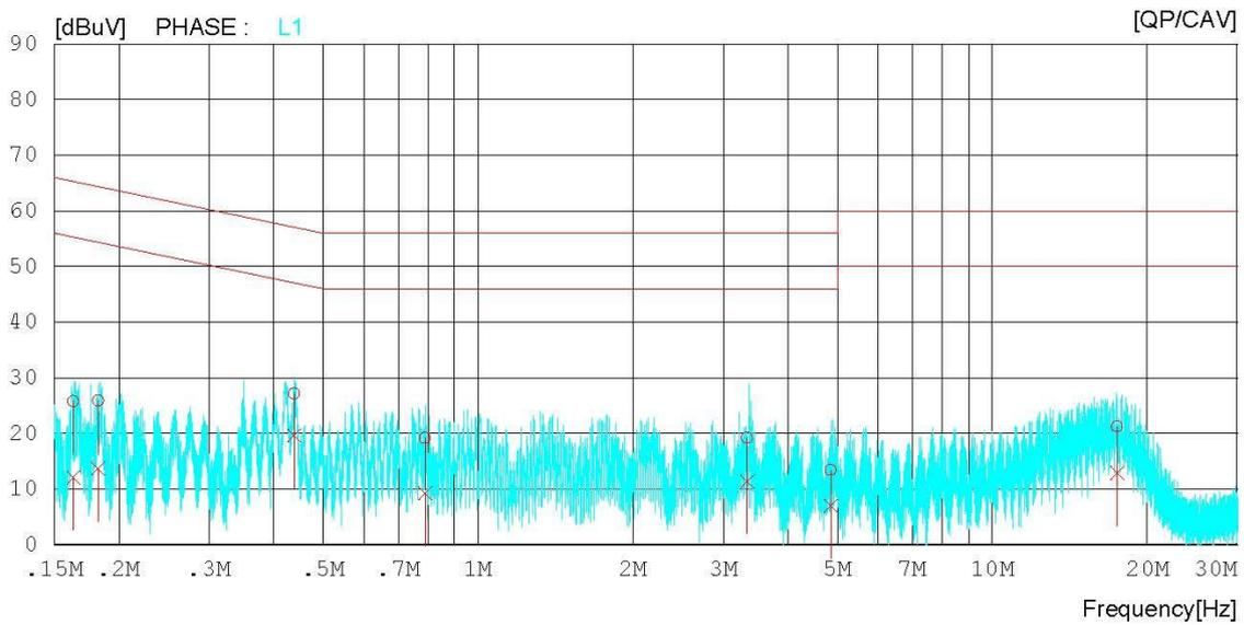
**AC Line Conducted Emissions (List) = TM 2 & Test Channel : Middle**
