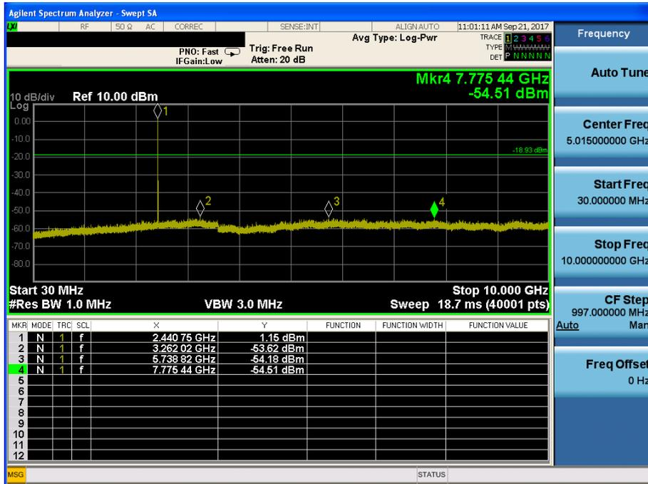
TM 2 Conducted Spurious Emissions 3 (Test Channel : Middle)
