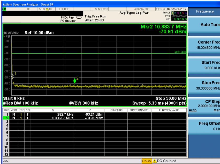
TM 1 Conducted Spurious Emissions 2 (Test Channel : Lowest)
