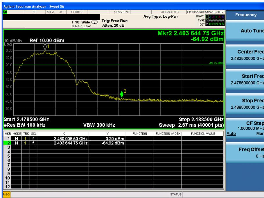
TM 2 Conducted Spurious Emissions 1 (Test Channel : Highest)
