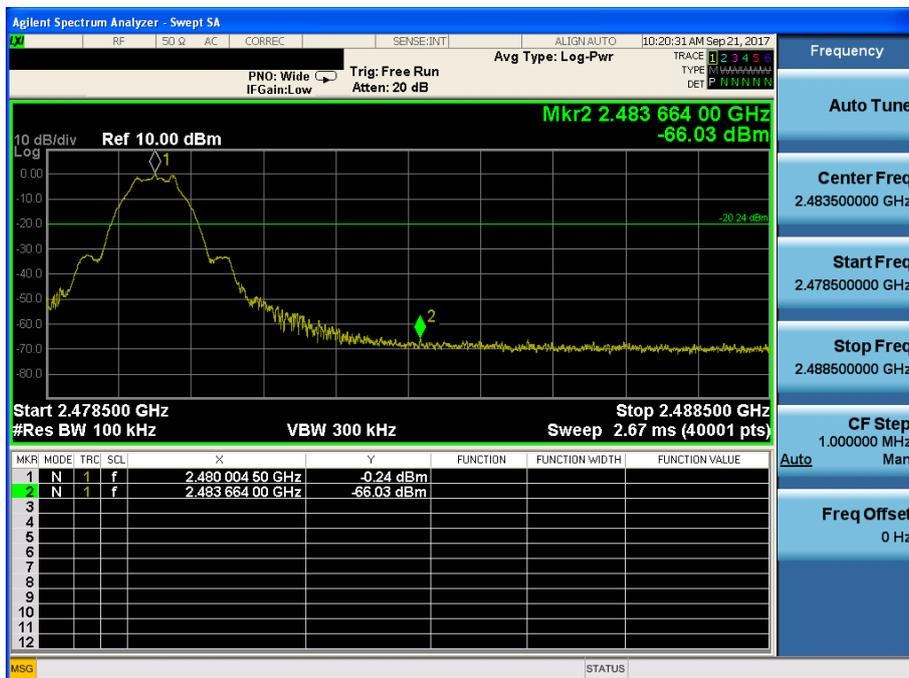
TM 1 Conducted Spurious Emissions 1 (Test Channel : Highest)
