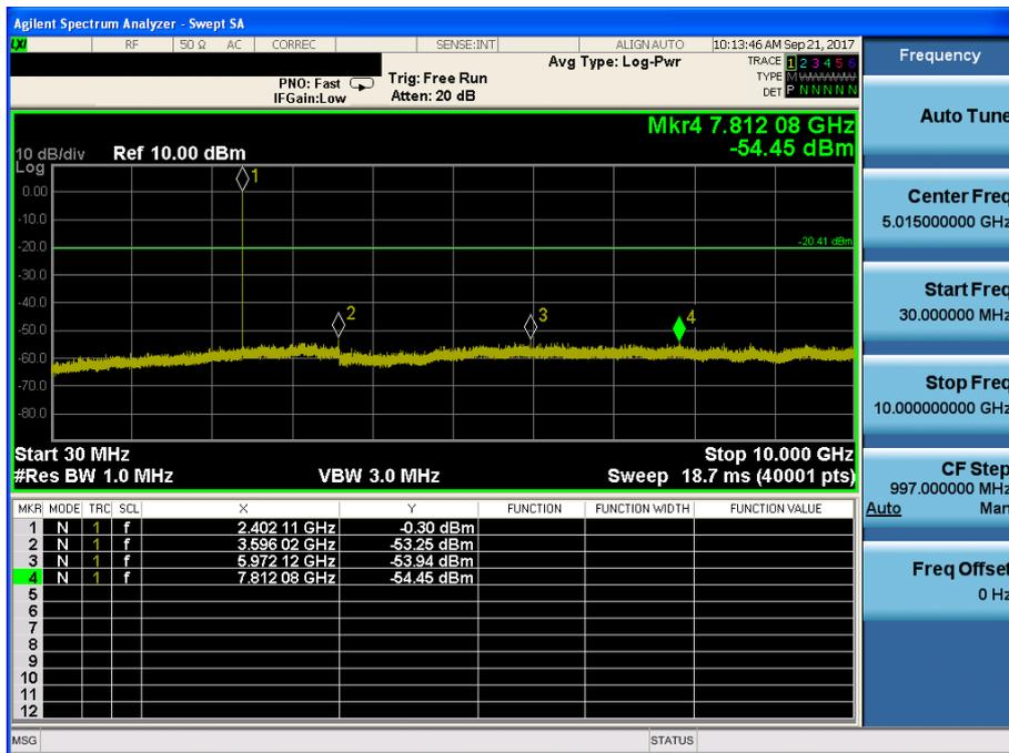
TM 1 Conducted Spurious Emissions 3 (Test Channel : Lowest)
