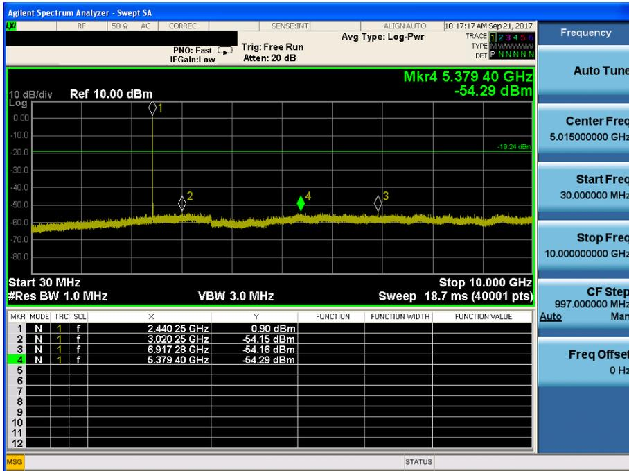
TM 1 Conducted Spurious Emissions 3 (Test Channel : Middle)
