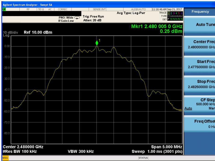
TM 2 High Band-edge (Test Channel : Highest)
