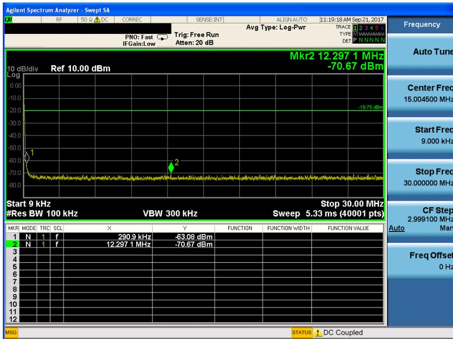
TM 2 Conducted Spurious Emissions 2 (Test Channel : Highest)
