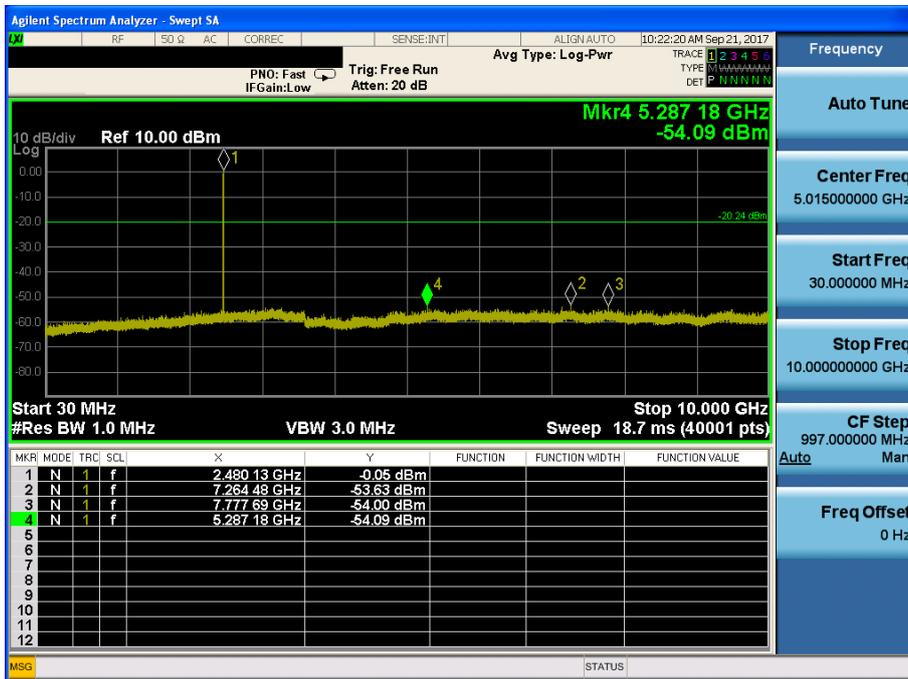
TM 1 Conducted Spurious Emissions 3 (Test Channel : Highest)
