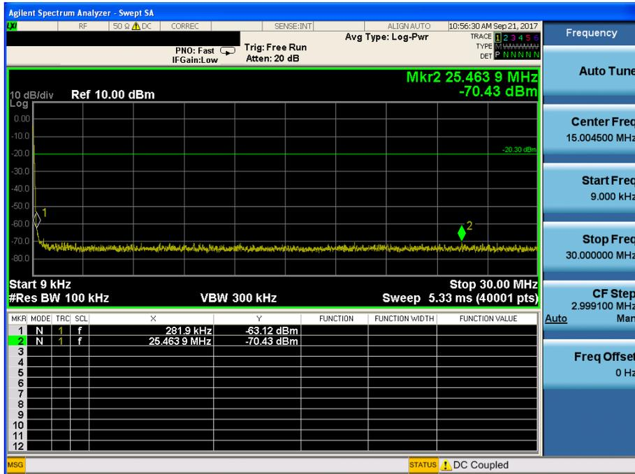
TM 2 Conducted Spurious Emissions 2 (Test Channel : Lowest)
