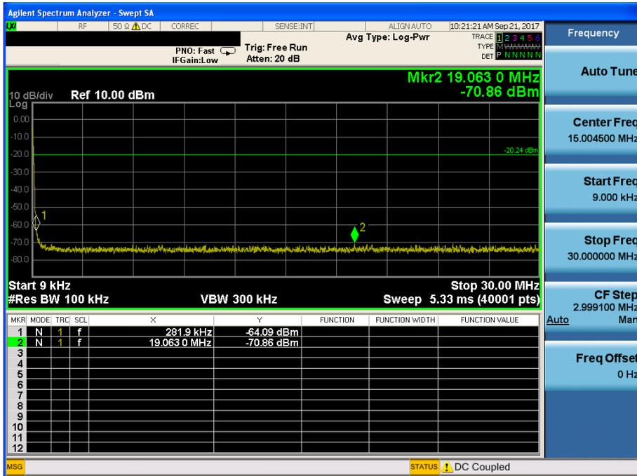
TM 1 Conducted Spurious Emissions 2 (Test Channel : Highest)
