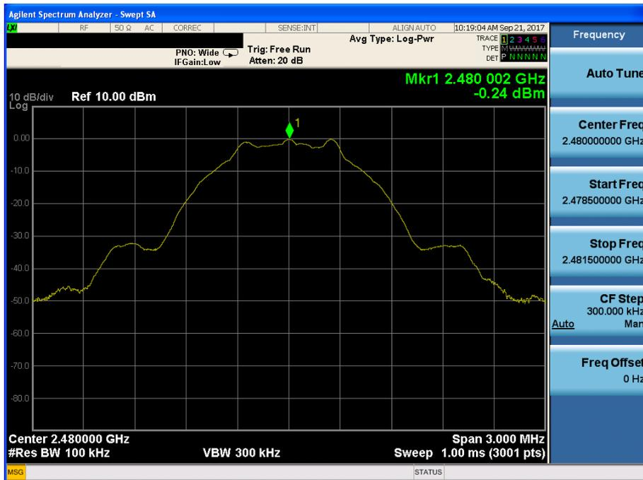
TM 1 High Band-edge (Test Channel : Highest)
