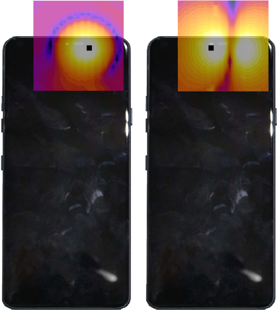
Figure 16-3 T-Coil Scan Overlay Magnetic Field Distributions
