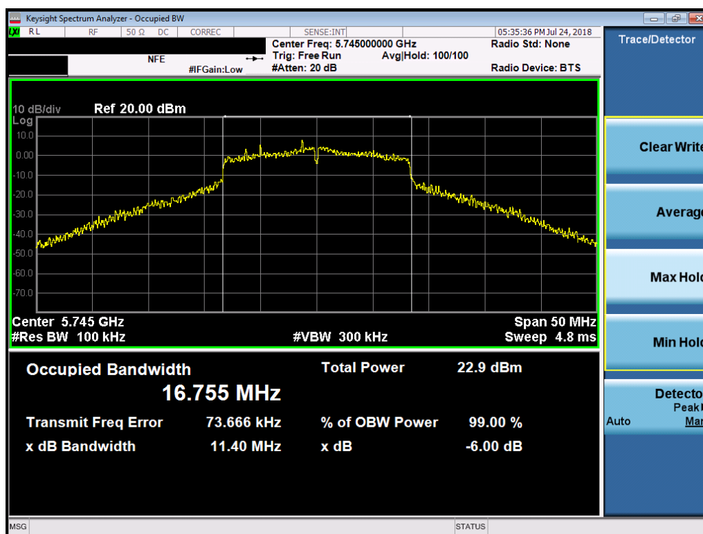
Plot 7-70. 6dB Bandwidth Plot SISO ANT2 (802.11a) (UNII Band 3) – Ch. 149)
