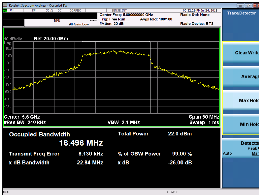
Plot 7-50. 26dB Bandwidth Plot SISO ANT2 (802.11a (UNII Band 2C) – Ch. 120)
