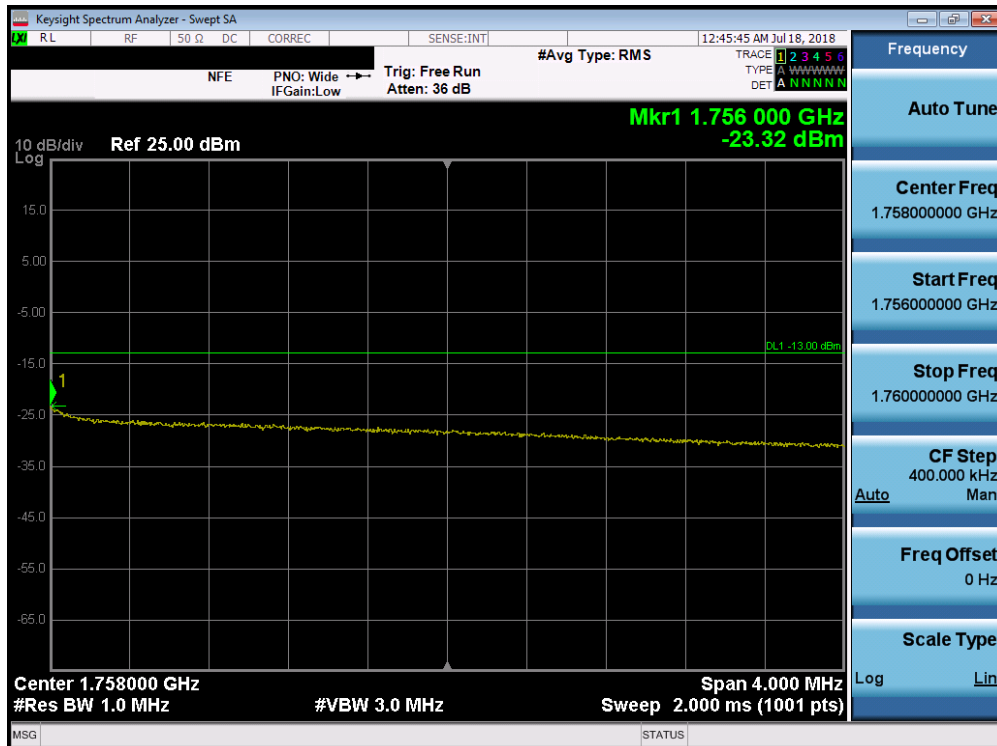
Plot 7-210. Upper Extended Band Edge Plot (Band 4 - 10.0MHz QPSK - Full RB Configuration)
