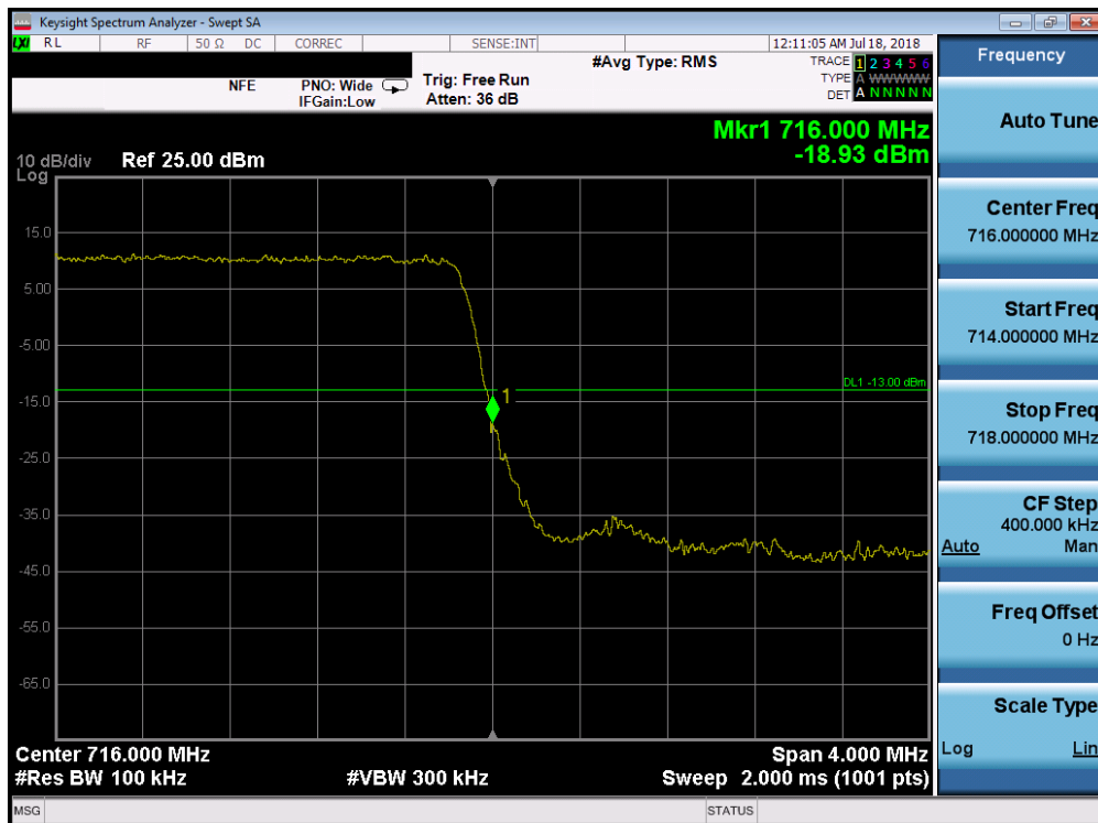
Plot 7-166. Upper Band Edge Plot (Band 12 - 3.0MHz QPSK - Full RB Configuration)
