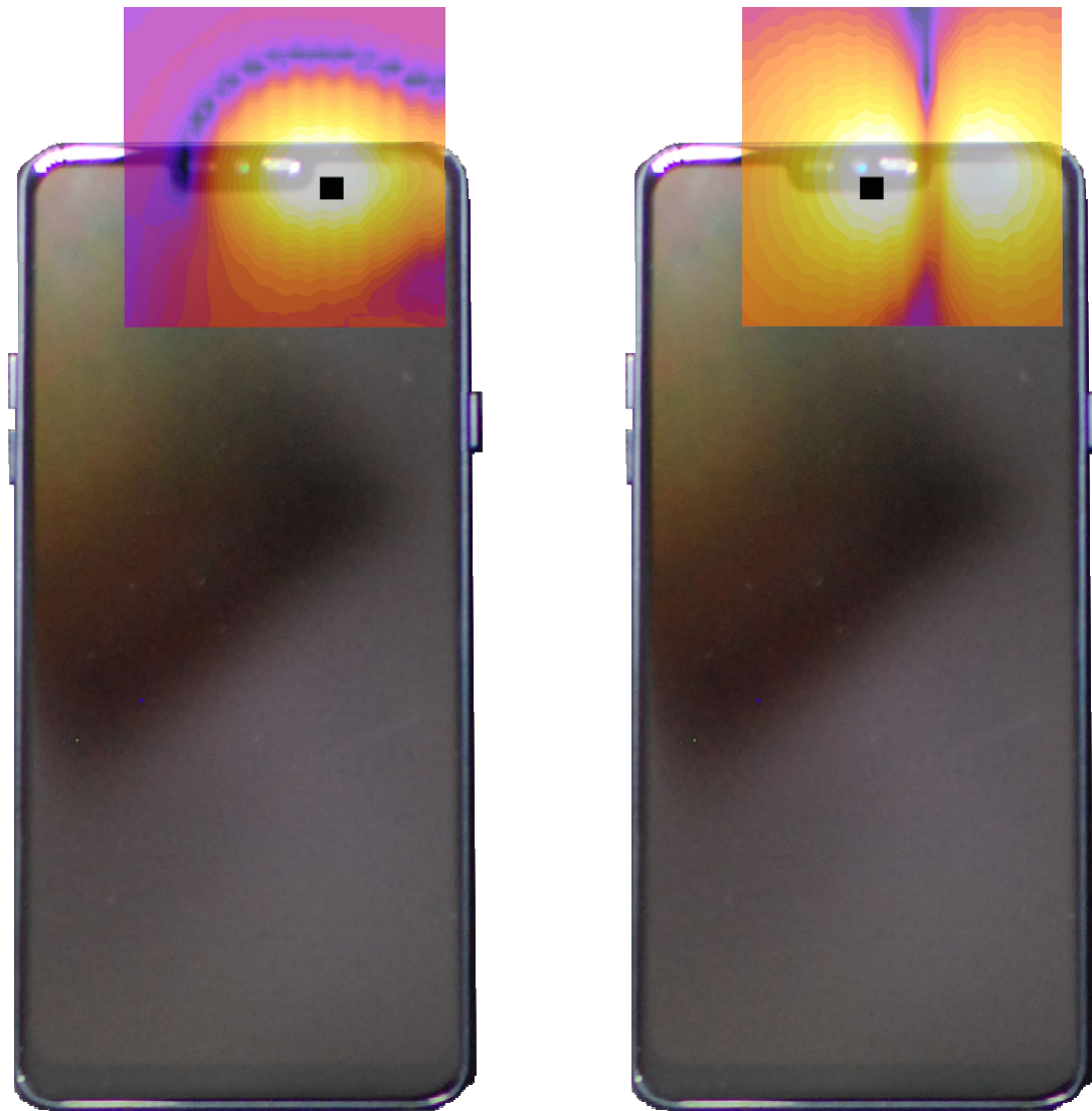
Figure 16-3 T-Coil Scan Overlay Magnetic Field Distributions
