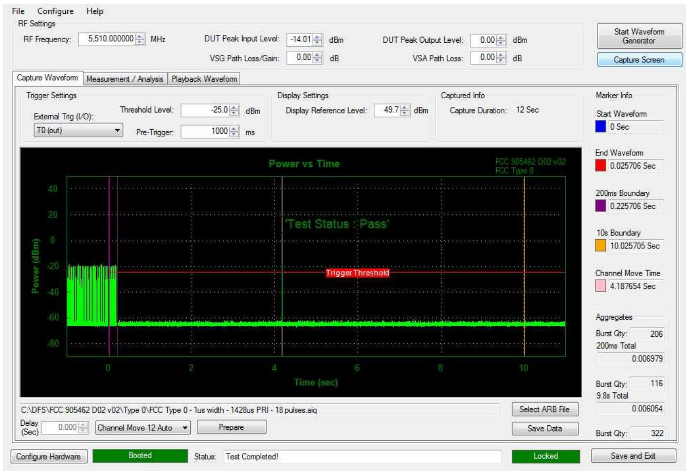
Figure 5-4. Band 2C Move Time and Aggregate Time
