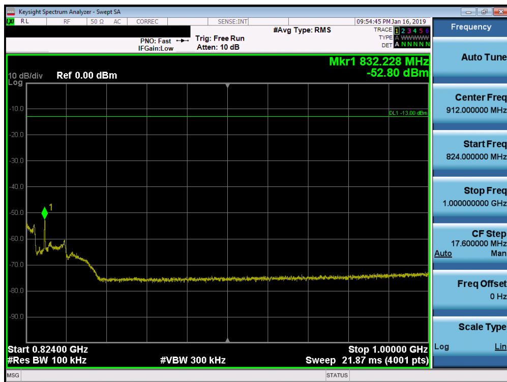
Plot 7-25. Conducted Spurious Plot (LTE Band 26, 10MHz QPSK – RB Size 1, RB Offset 0 – Mid Channel)
