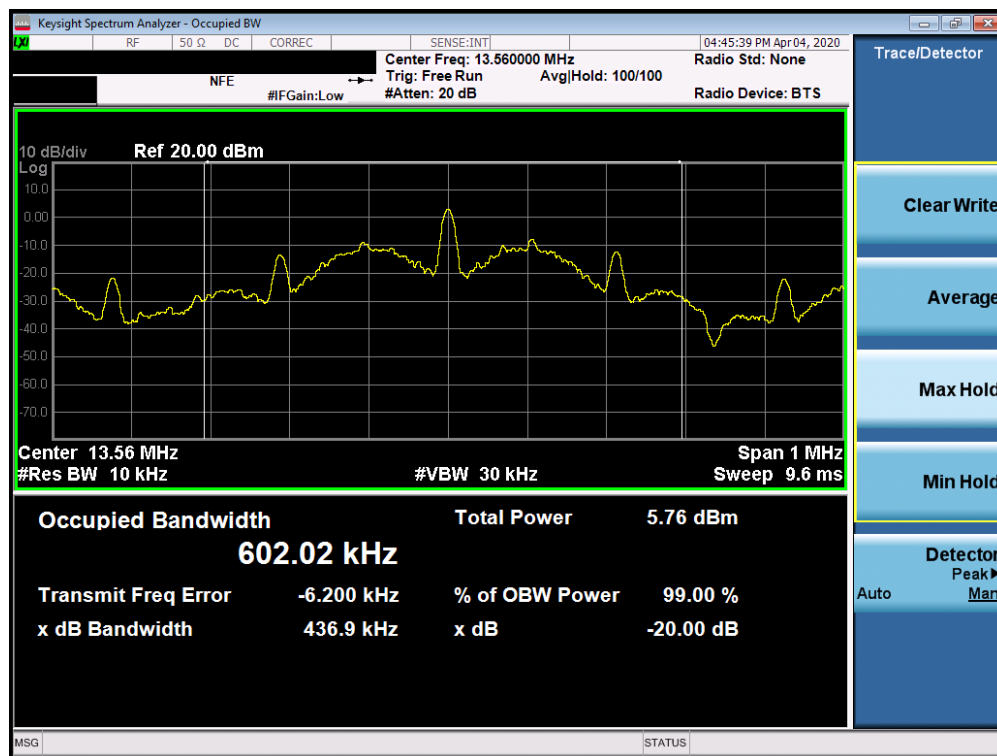
Figure 7-2. Occupied Bandwidth Plot
