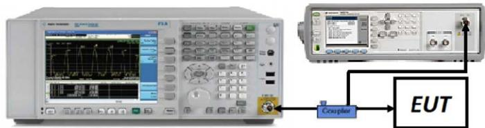
**Figure 7-2. Test Instrument & Measurement Setup**
