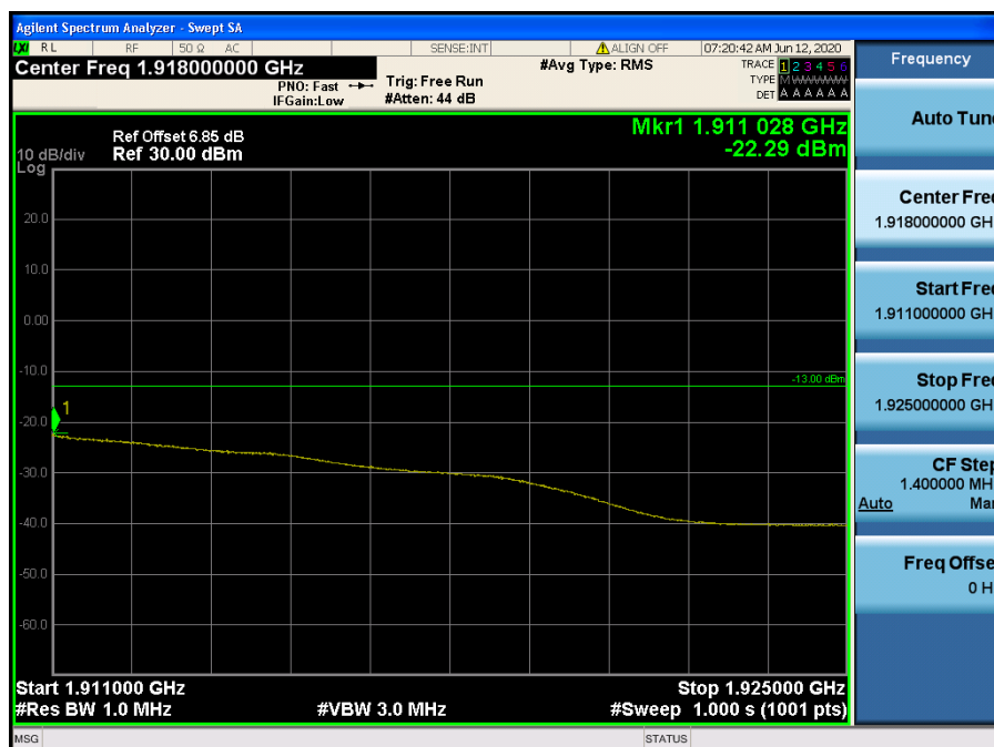
LTE Band 2 / 15 MHz / 16QAM - RB Size/Offset (36/39)
