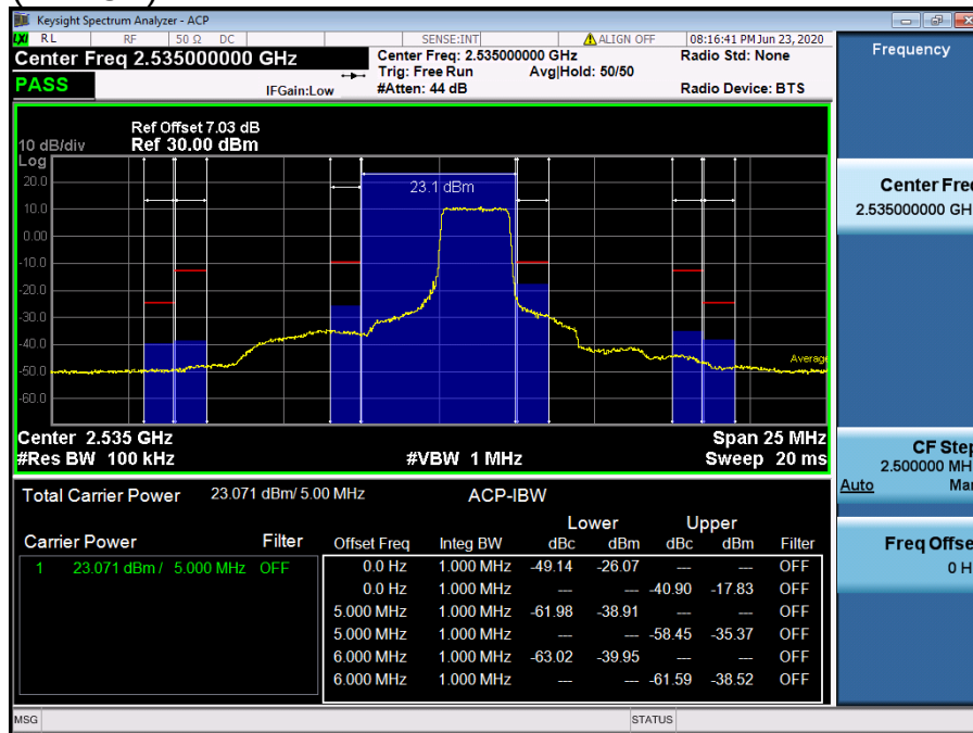
LTE Band 7 / 5 MHz / QPSK - RB Size/Offset (12/13)
