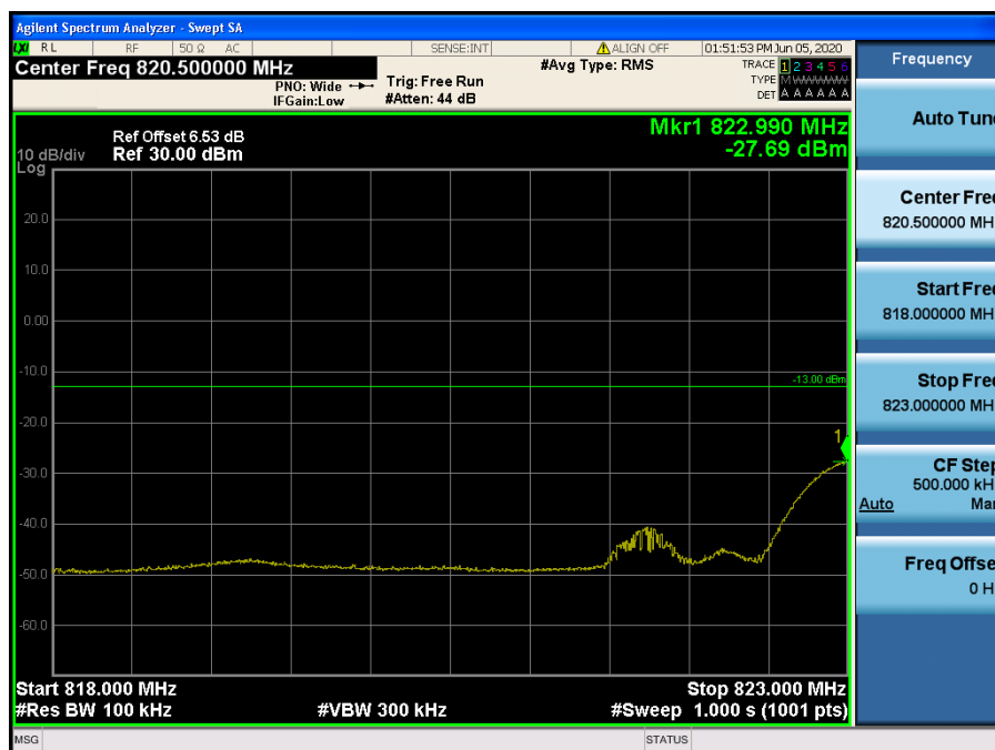
LTE Band 5 / 3MHz / 16QAM - RB Size/Offset (1/0)
