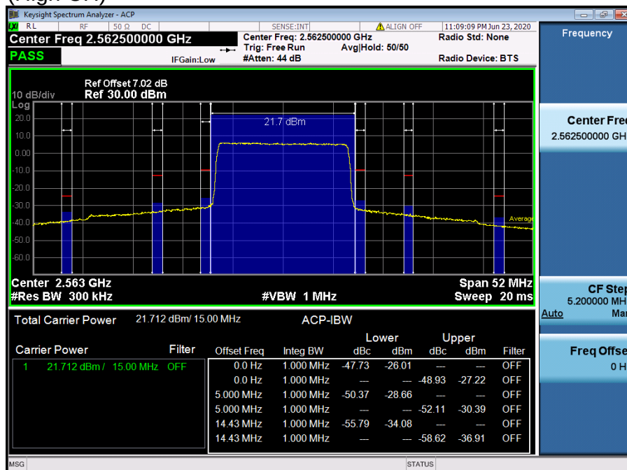
LTE Band 7 / 15 MHz / 16QAM - RB Size/Offset (75/0)
