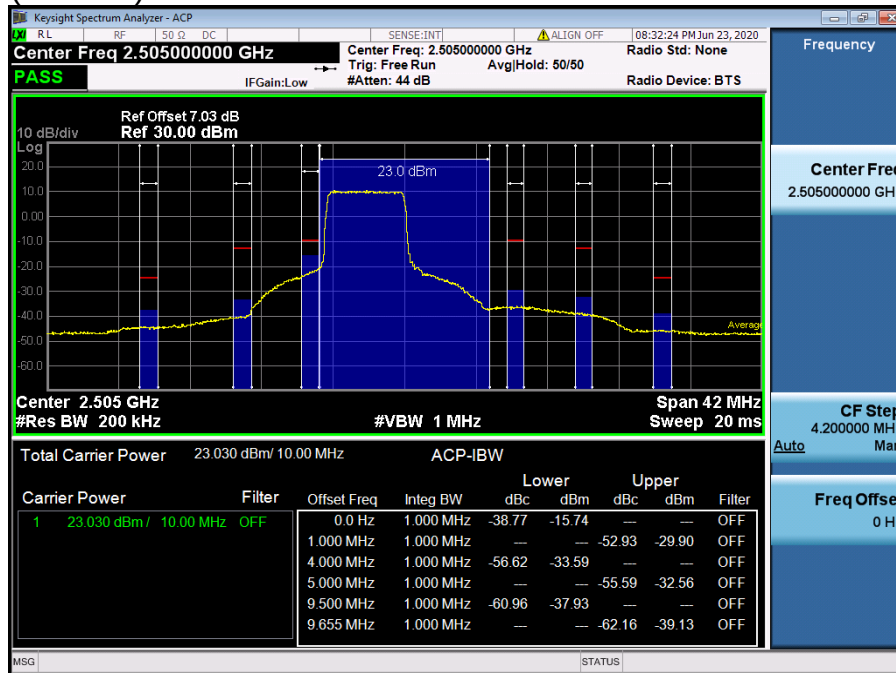
LTE Band 7 / 10 MHz / QPSK - RB Size/Offset (25/0)
