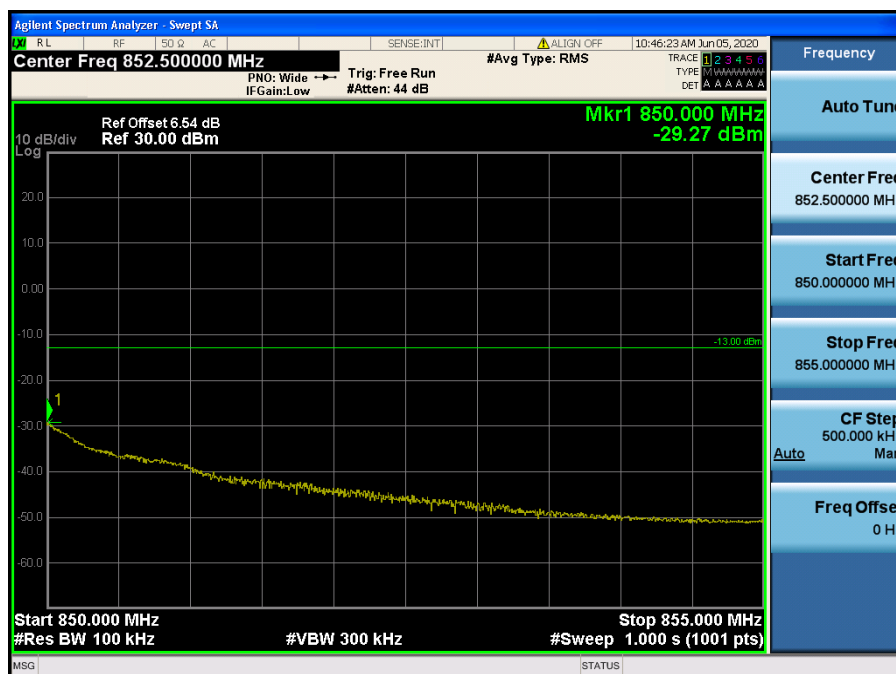
LTE Band 5 / 1.4 MHz / QPSK - RB Size/Offset (6/0)
