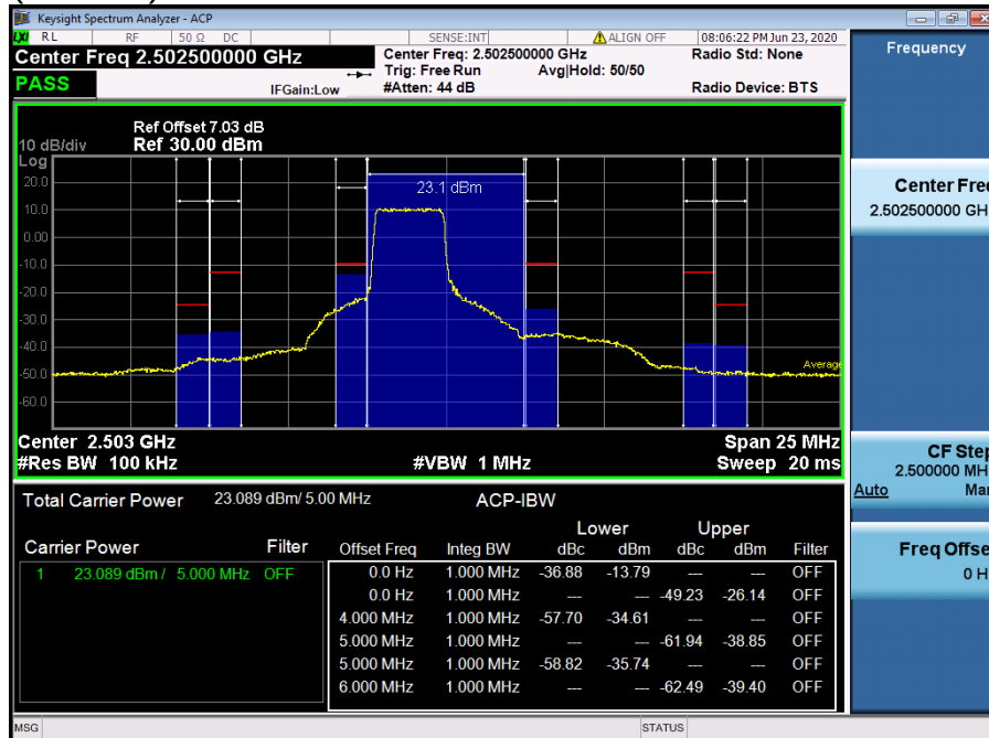
LTE Band 7 / 5 MHz / QPSK - RB Size/Offset (12/0)
