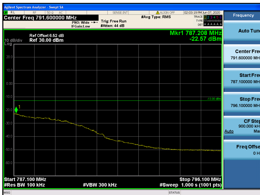
LTE Band 13 / 10 MHz / QPSK - RB Size/Offset (25/25)
