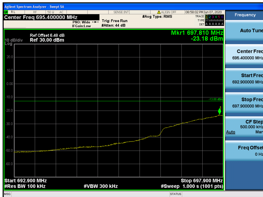
LTE Band 12 / 3MHz / QPSK - RB Size/Offset (15/0)
