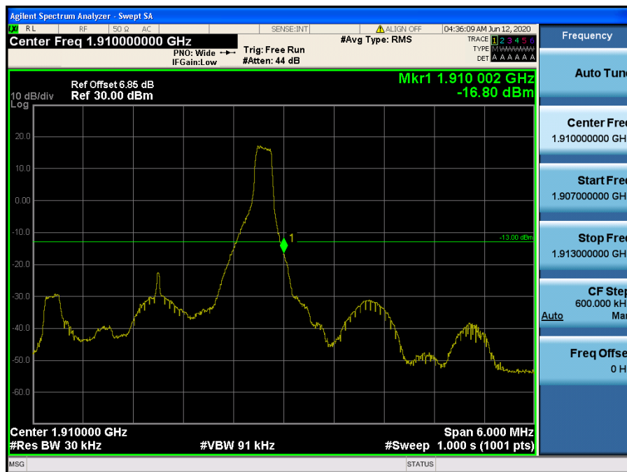
LTE Band 2 / 3MHz / 16QAM - RB Size/Offset (1/14)
