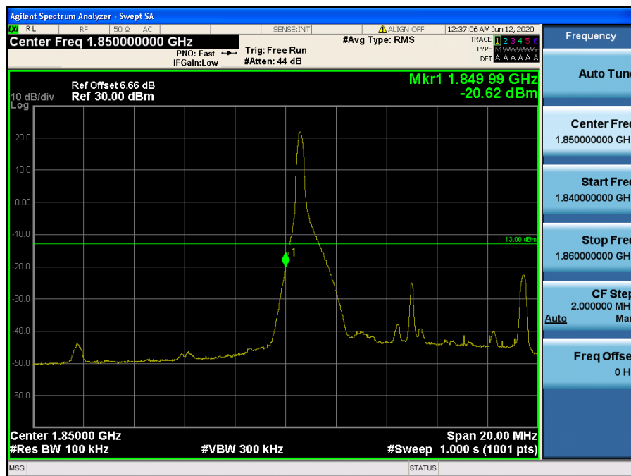
LTE Band 2 / 10 MHz / QPSK - RB Size/Offset (1/0)
