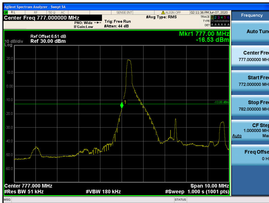
LTE Band 13 / 5 MHz / 16QAM - RB Size/Offset (1/0)
