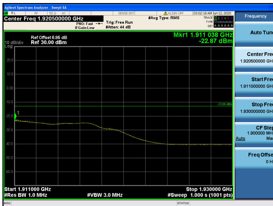
LTE Band 2 / 20 MHz / QPSK - RB Size/Offset (50/50)
