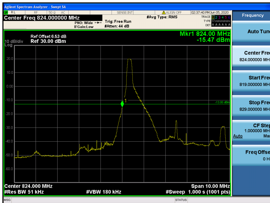
LTE Band 5 / 5 MHz / 16QAM- RB Size/Offset (1/0)
