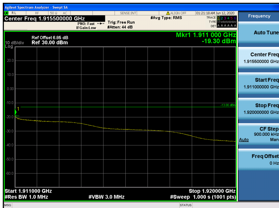
LTE Band 2 / 10 MHz / QPSK- RB Size/Offset (25/25)
