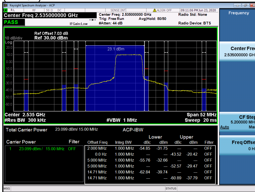
LTE Band 7 / 15 MHz / QPSK - RB Size/Offset (36/39)
