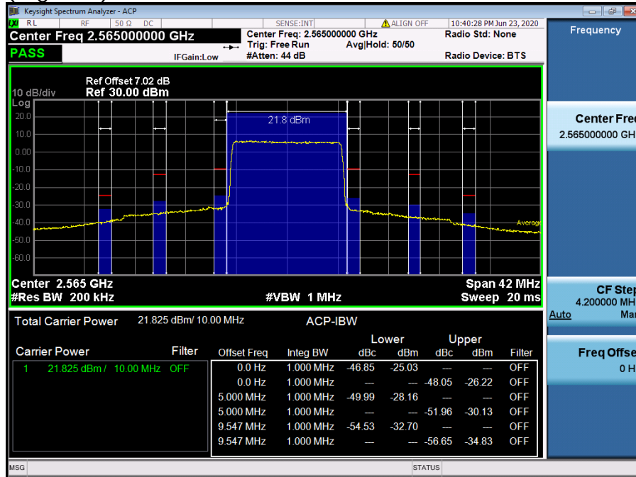
LTE Band 7 / 10 MHz / 16QAM - RB Size/Offset (50/0)
