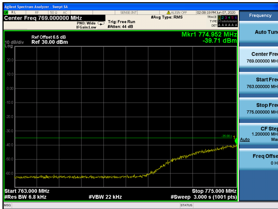
LTE Band 13 / 10 MHz / QPSK - RB Size/Offset (50/0)
