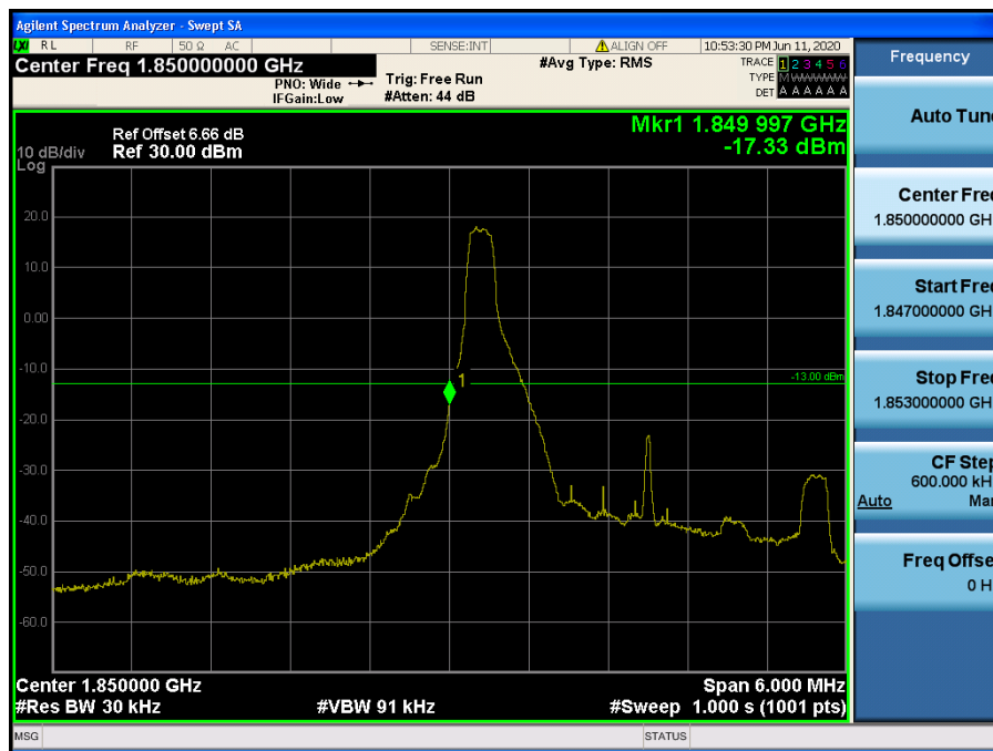
LTE Band 2 / 3MHz / QPSK - RB Size/Offset (1/0)
