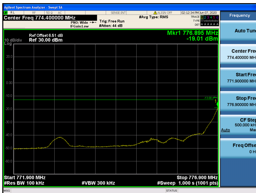
LTE Band 13 / 5 MHz / 16QAM - RB Size/Offset (1/0)
