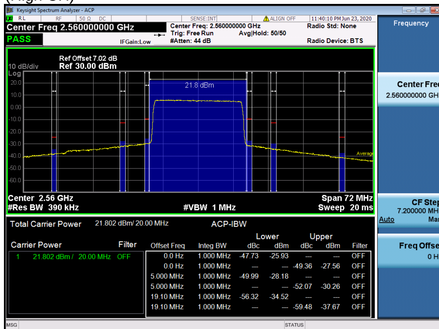
LTE Band 7 / 20 MHz / 16QAM - RB Size/Offset (100/0)
