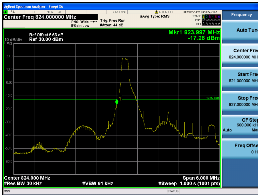
LTE Band 5 / 3MHz / 16QAM - RB Size/Offset (1/0)
