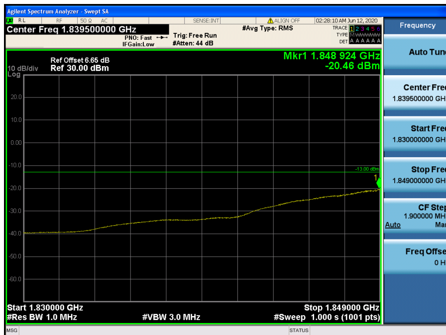
LTE Band 2 / 20 MHz / QPSK - RB Size/Offset (50/0)
