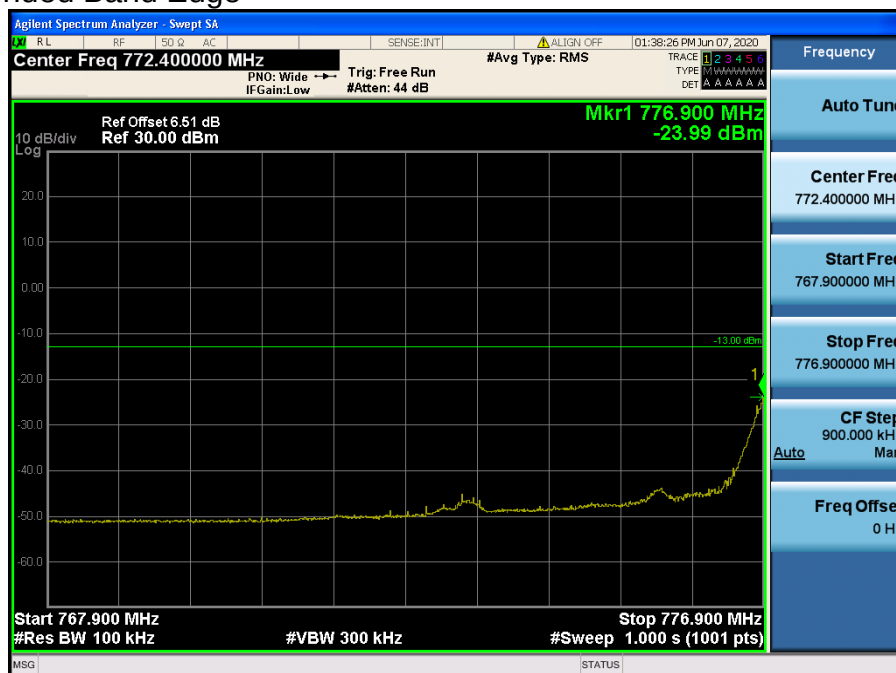
LTE Band 13 / 10 MHz / QPSK - RB Size/Offset (1/0)
