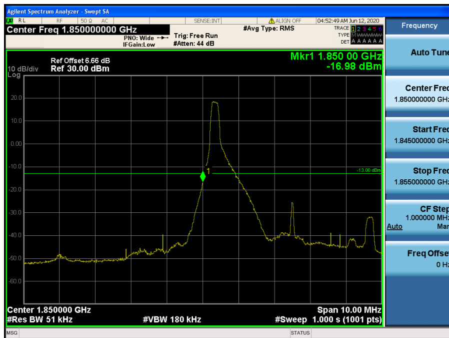
LTE Band 2 / 5 MHz / 16QAM - RB Size/Offset (1/0)
