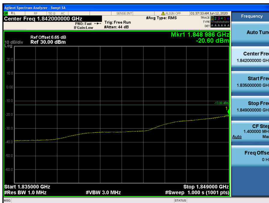
LTE Band 2 / 15 MHz / QPSK - RB Size/Offset (36/0)
