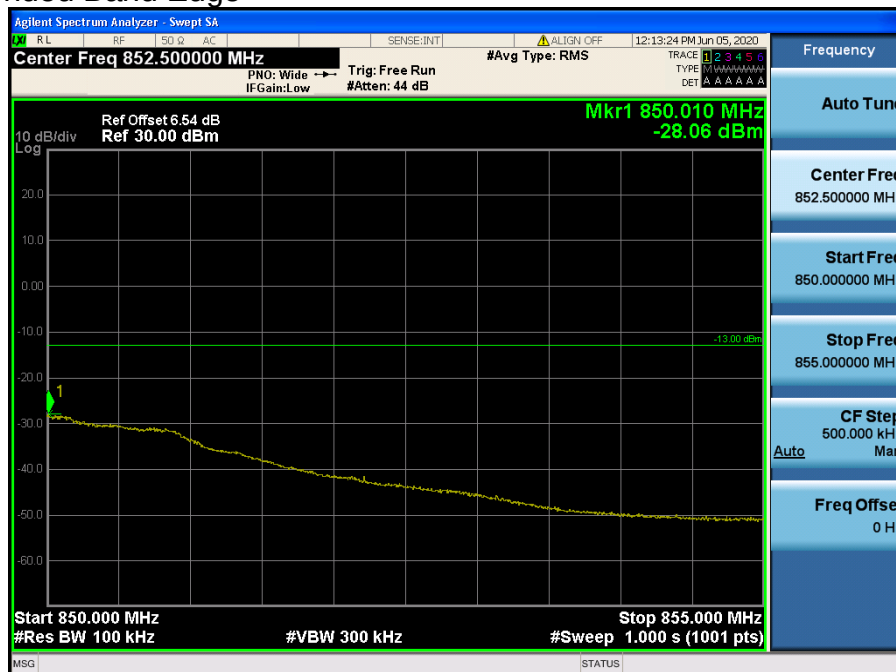
LTE Band 5 / 5 MHz / QPSK - RB Size/Offset (12/13)
