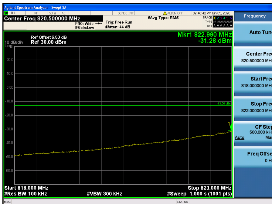
LTE Band 5 / 5 MHz / 16QAM - RB Size/Offset (12/0)
