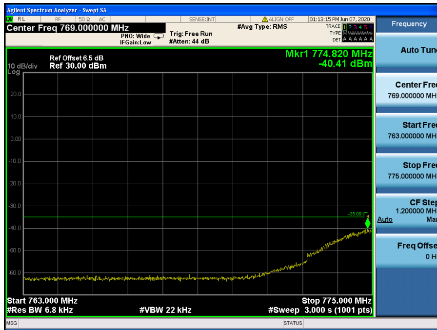
LTE Band 13 / 5 MHz / QPSK - RB Size/Offset (25/0)
