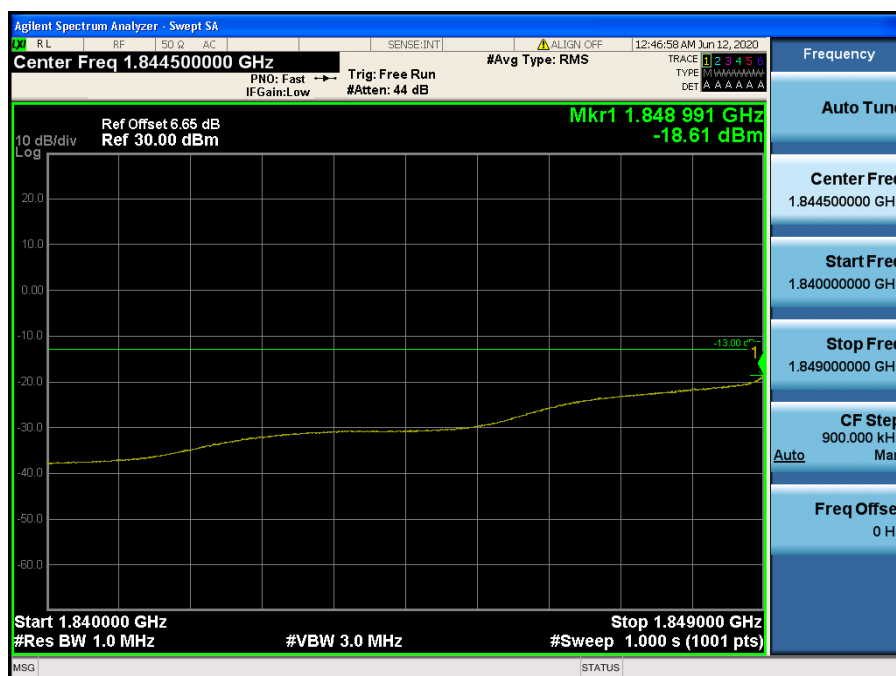
LTE Band 2 / 10 MHz / QPSK - RB Size/Offset (25/0)
