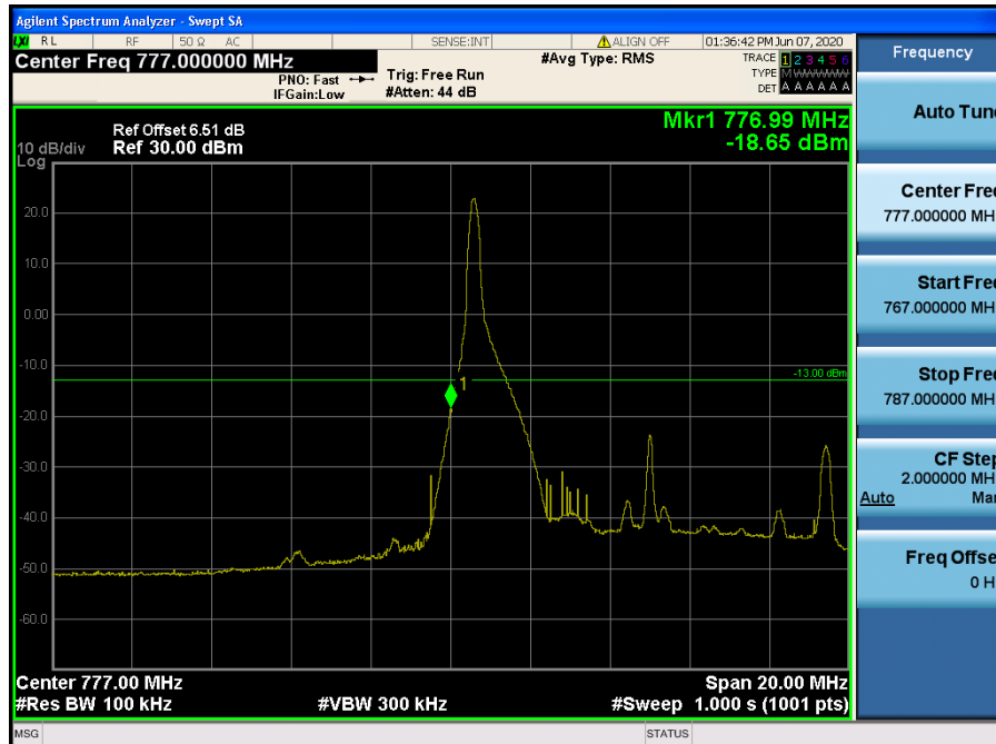
LTE Band 13 / 10 MHz / QPSK - RB Size/Offset (1/0)
