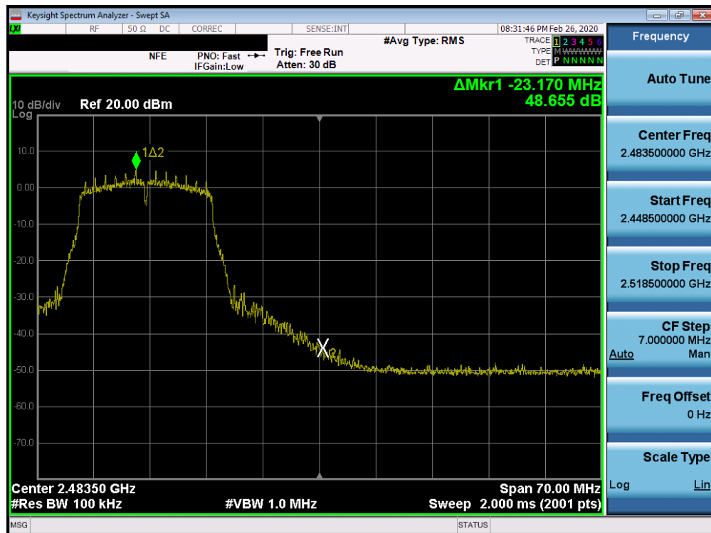
Plot 7-22. Band Edge Plot (802.11g – Ch. 11)
