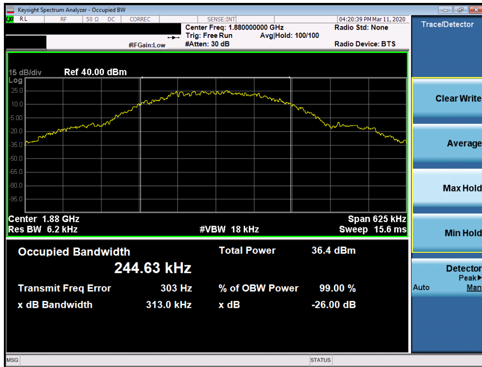
Plot 7-3. Occupied Bandwidth Plot (PCS GPRS Mode)
