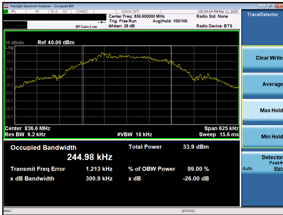
Plot 7-2. Occupied Bandwidth Plot (EDGE850 Mode)
