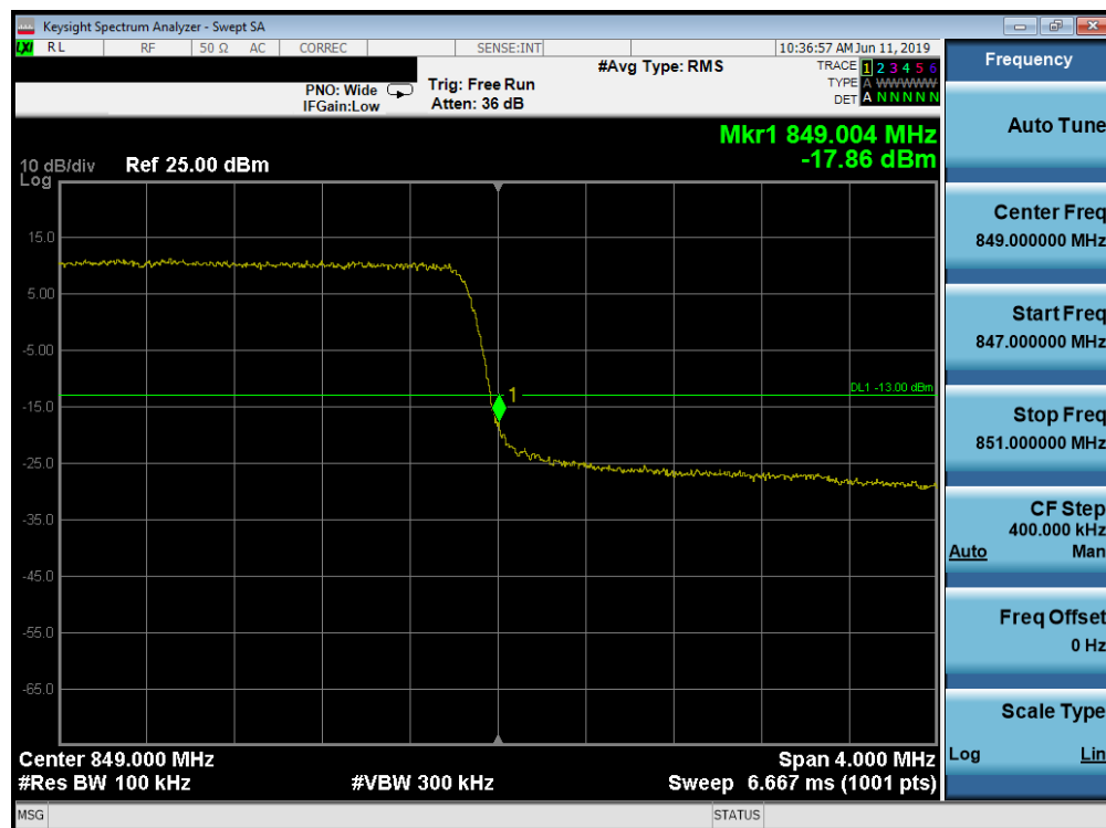
Plot 7-96. Upper Band Edge Plot (Band 5 - 3.0MHz QPSK - Full RB Configuration)
