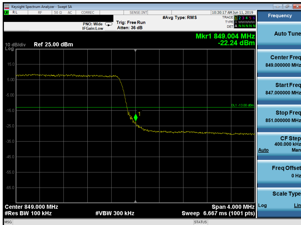
Plot 7-98. Upper Band Edge Plot (Band 5 - 5.0MHz QPSK - Full RB Configuration)
