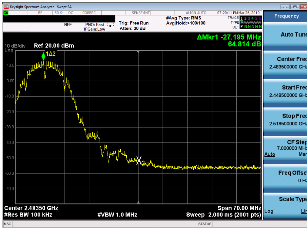
Plot 7-23. Band Edge Plot (802.11b – Ch. 10)
