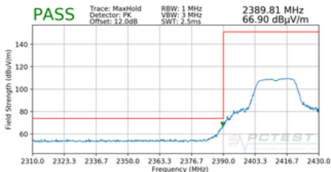
Plot 7-48. Radiated Restricted Lower Band Edge Measurement (Peak)
