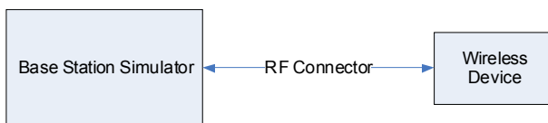
Figure 9-2 Power Measurement Setup
