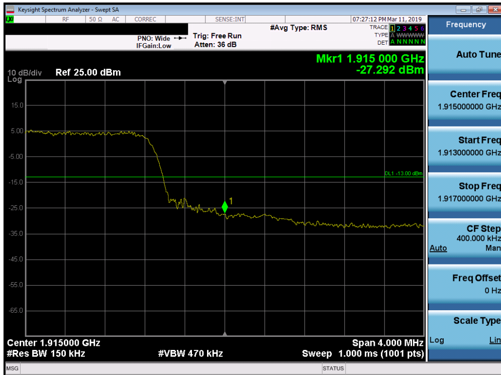
Plot 7-257. Upper Band Edge Plot (Band 25 - 15.0MHz QPSK - Full RB Configuration)
