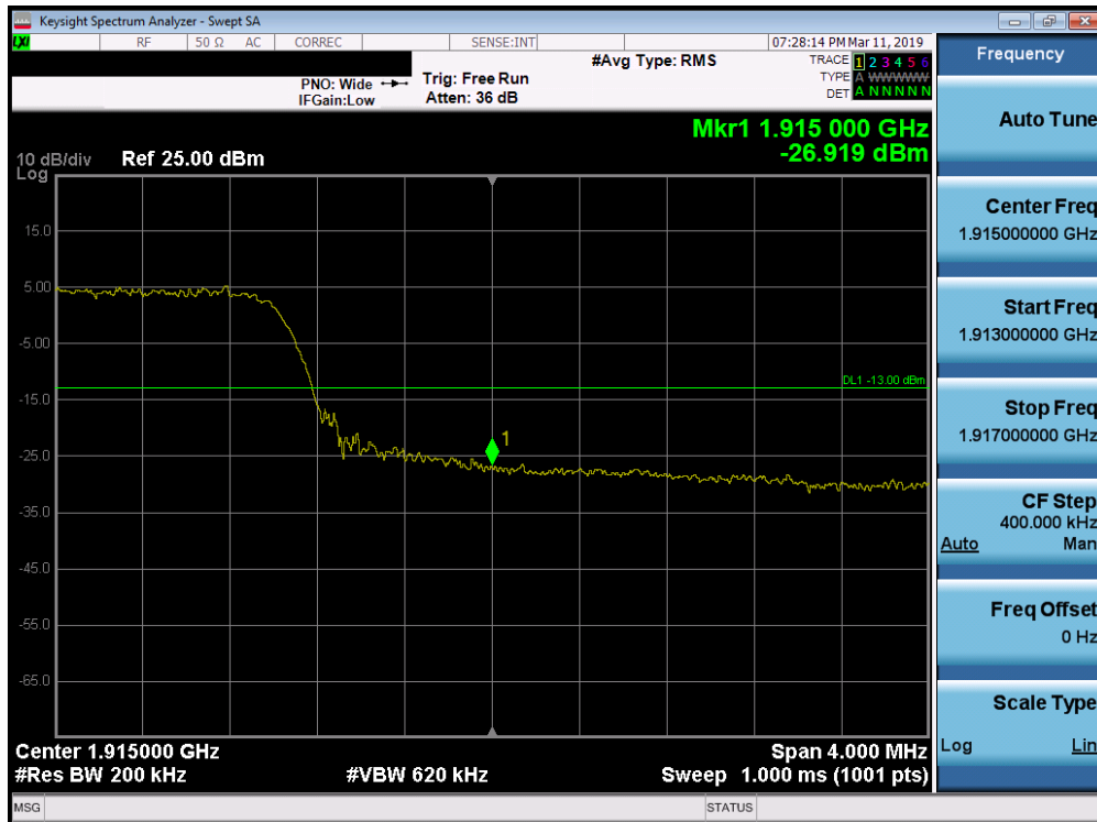
Plot 7-263. Upper Band Edge Plot (Band 25 - 20.0MHz QPSK - Full RB Configuration)
