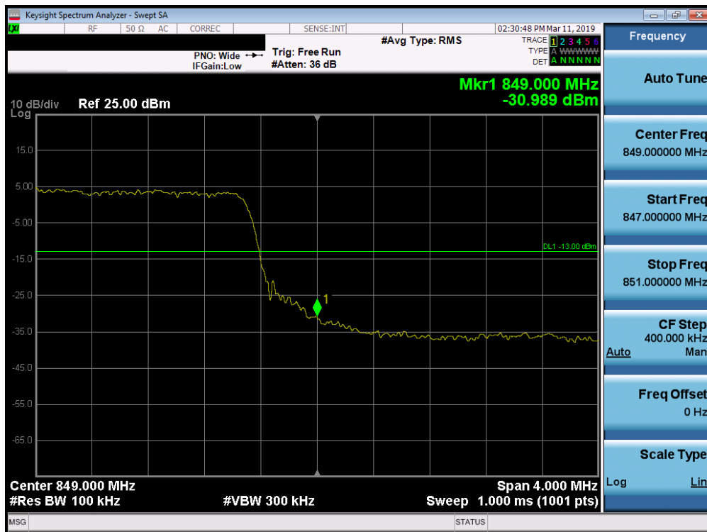
Plot 7-190. Upper Band Edge Plot (Band 26/5 - 10.0MHz QPSK - Full RB Configuration)
