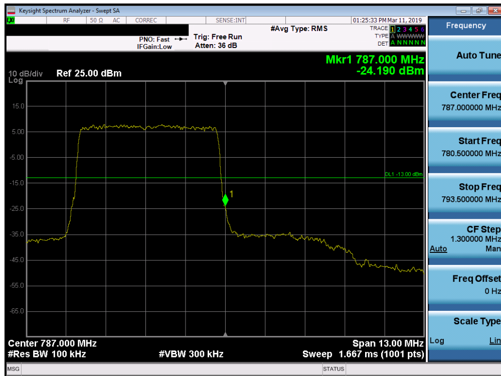
Plot 7-177. Upper Band Edge Plot (Band 13 - 5.0MHz QPSK - Full RB Configuration)
