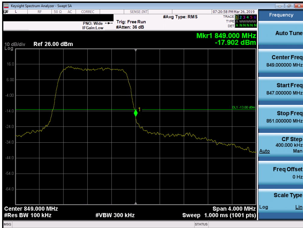
Plot 7-184. Upper Band Edge Plot (Band 26/5 - 1.4MHz QPSK - Full RB Configuration)
