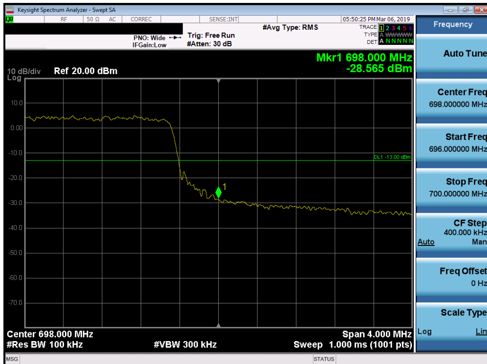
Plot 7-160. Upper Band Edge Plot (Band 71 - 10.0MHz QPSK - Full RB Configuration)
