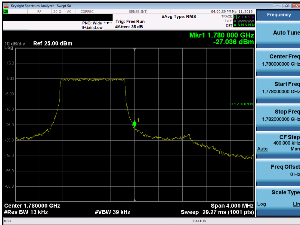
Plot 7-197. Upper Band Edge Plot (Band 66 - 1.4MHz QPSK - Full RB Configuration)
