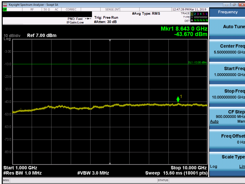
Plot 7-105. Conducted Spurious Plot (Band 12/17 - 10.0MHz QPSK - RB Size 1, RB Offset 0 - Low Channel)
