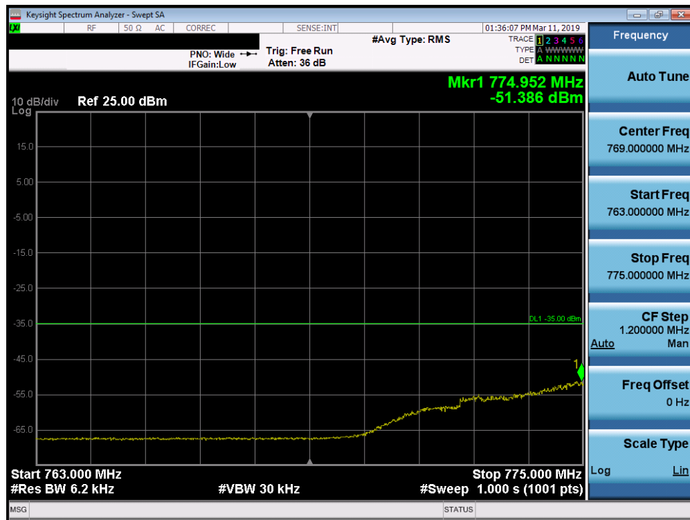
Plot 7-180. Lower Emission Mask Plot (Band 13 - 10.0MHz QPSK - Full RB Configuration)
