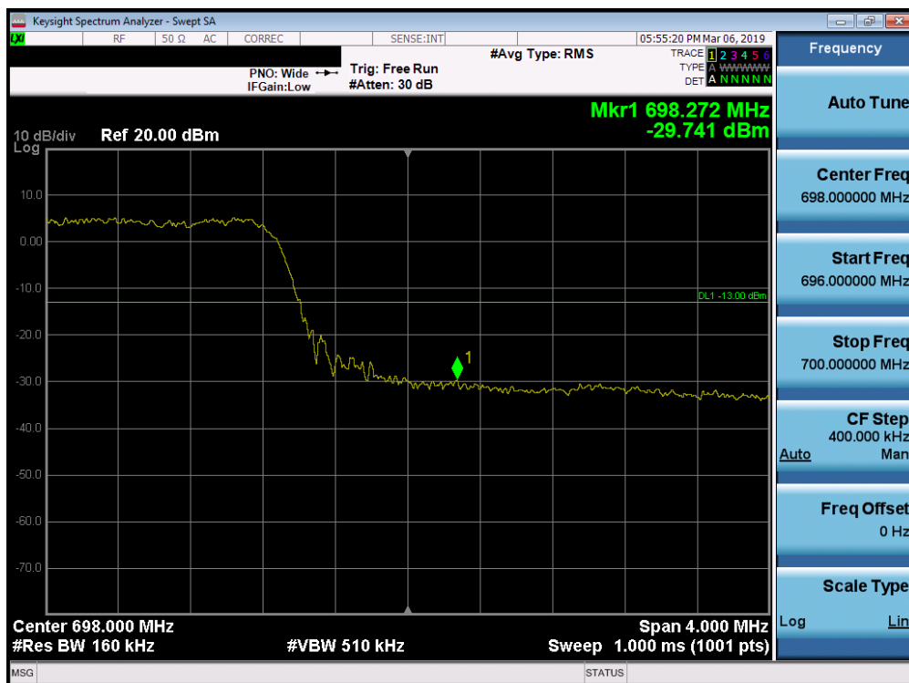
Plot 7-162. Upper Band Edge Plot (Band 71 - 15.0MHz QPSK - Full RB Configuration)
