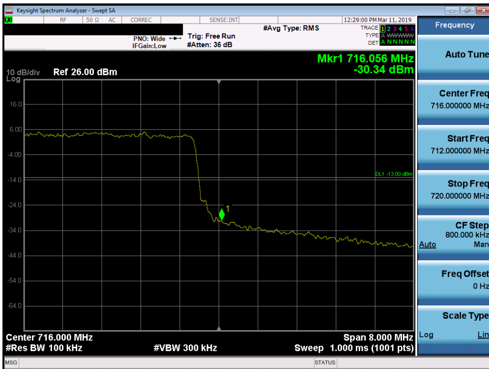
Plot 7-174. Upper Band Edge Plot (Band 12/17 - 10.0MHz QPSK - Full RB Configuration)
