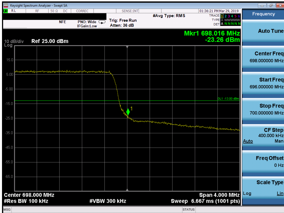
Plot 7-158. Upper Band Edge Plot (Band 71 - 5.0MHz QPSK - Full RB Configuration)
