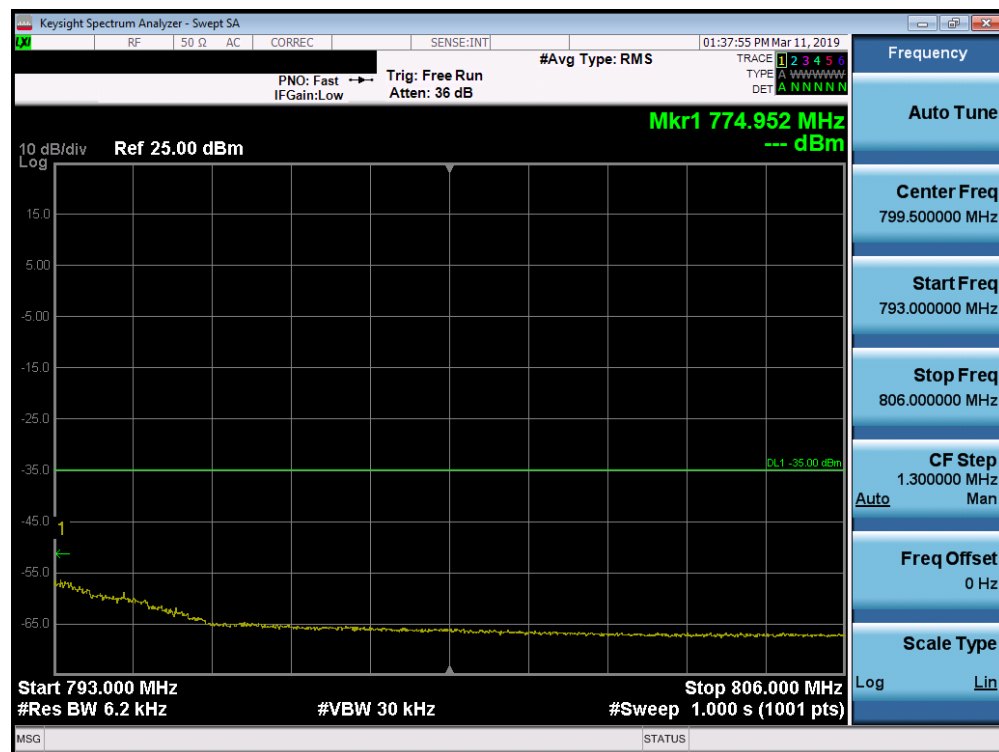
Plot 7-182. Upper Emission Mask Plot (Band 13 - 10.0MHz QPSK - Full RB Configuration)
