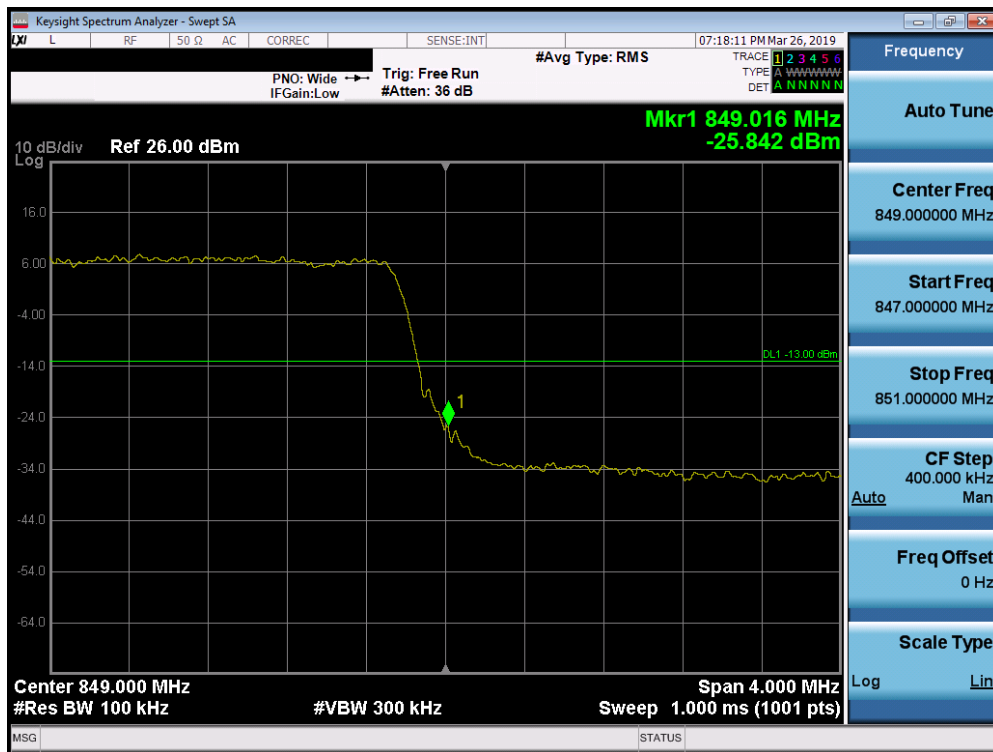
Plot 7-188. Upper Band Edge Plot (Band 26/5 - 5.0MHz QPSK - Full RB Configuration)
