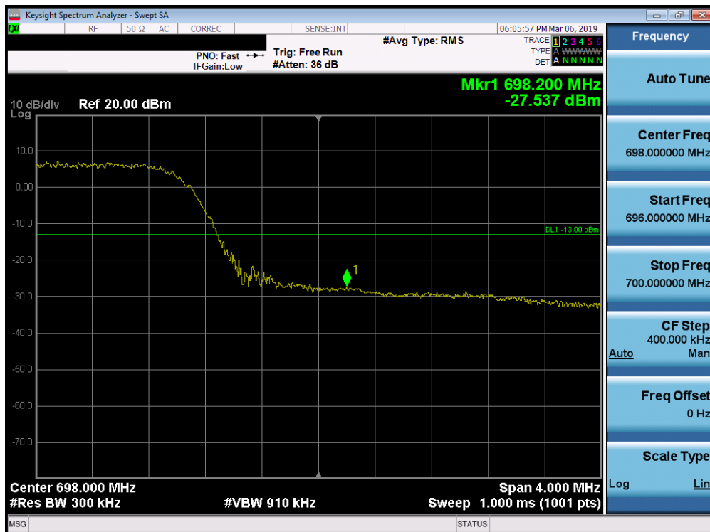
Plot 7-164. Upper Band Edge Plot (Band 71 - 20.0MHz QPSK - Full RB Configuration)
