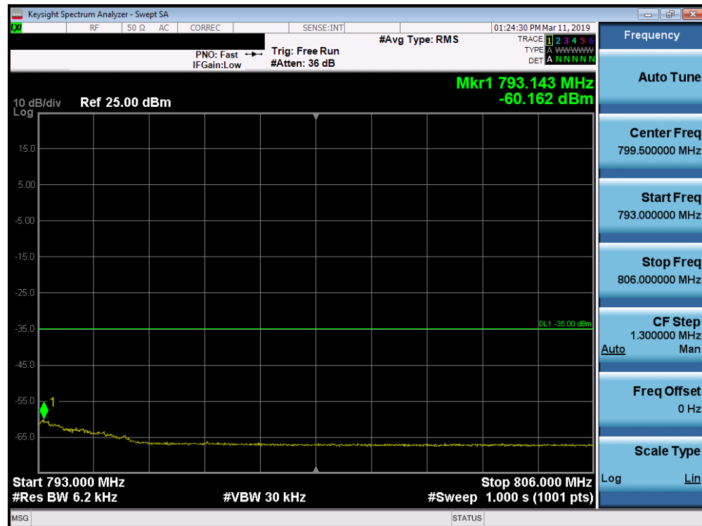
Plot 7-178. Upper Emission Mask Plot (Band 13 - 5.0MHz QPSK - Full RB Configuration)
