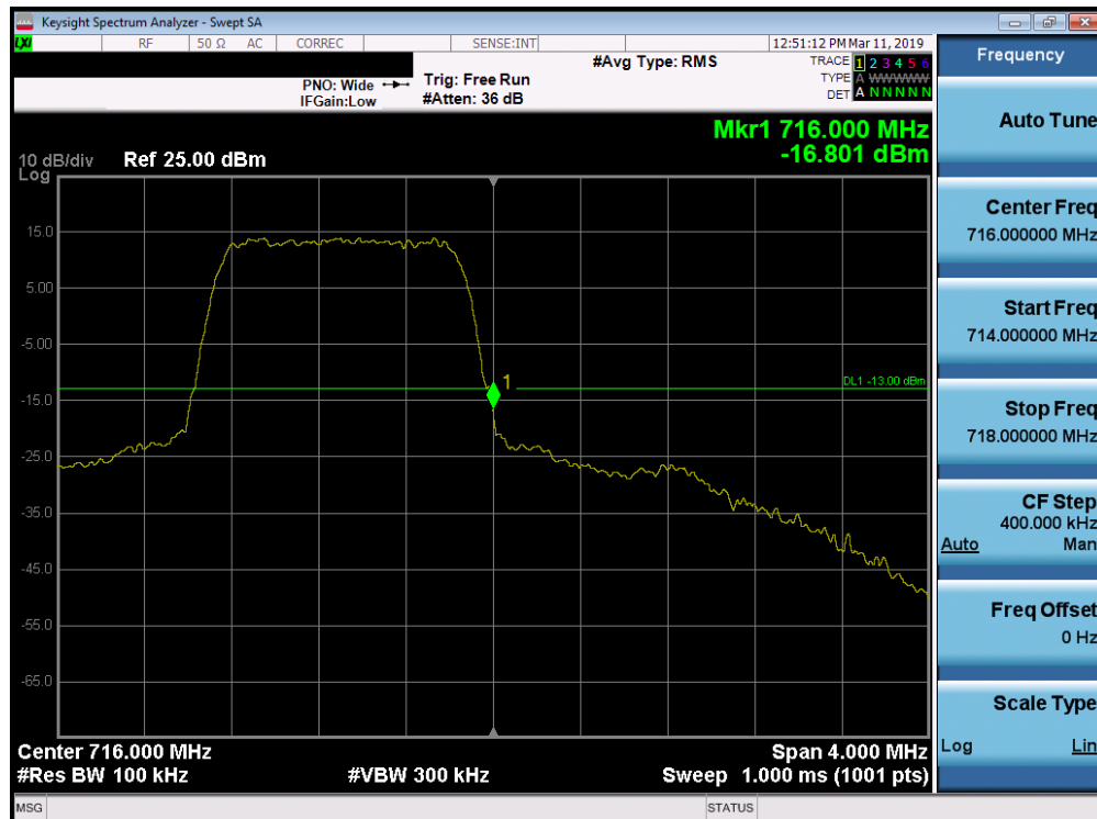
Plot 7-166. Upper Band Edge Plot (Band 12 - 1.4MHz QPSK - Full RB Configuration)
