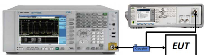
Figure 7-5. Test Instrument & Measurement Setup
