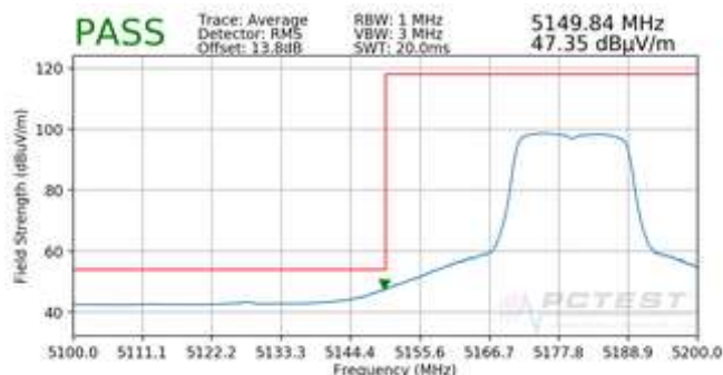
Plot 7-7. Radiated Lower Band Edge Plot (Average – UNII Band 1)
