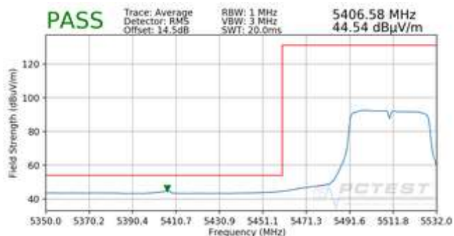
Plot 7-27. Radiated Lower Band Edge Plot (Average – UNII Band 2C)
