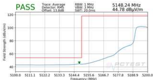
Plot 7-9. Radiated Lower Band Edge Plot (Average – UNII Band 1)
