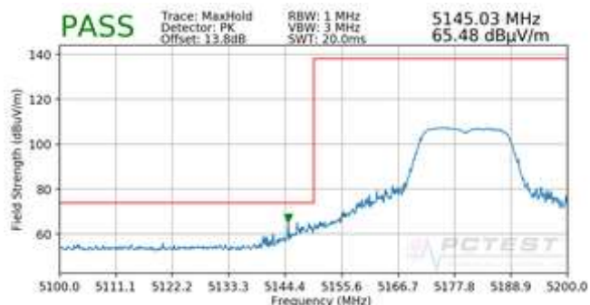
Plot 7-8. Radiated Lower Band Edge Plot (Peak – UNII Band 1)
