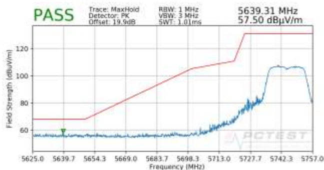
Plot 7-21. Radiated Upper Band Edge Plot (Peak – UNII Band 2C)
