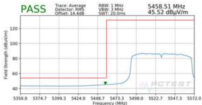
Plot 7-36. Radiated Lower Band Edge Plot (Average – UNII Band 2C)
