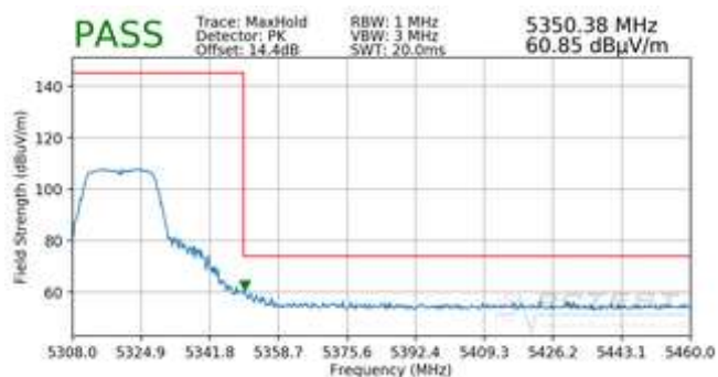
Plot 7-14. Radiated Upper Band Edge Plot (Peak – UNII Band 2A)
