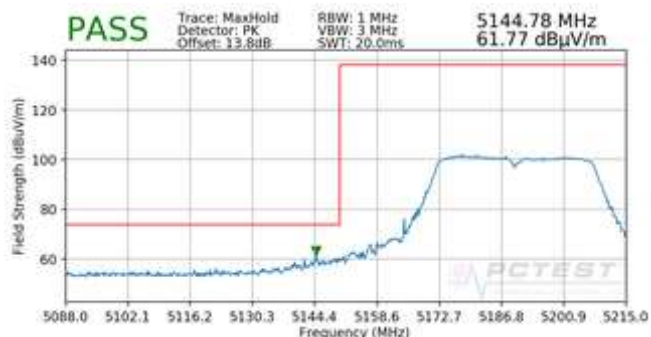
Plot 7-24. Radiated Lower Band Edge Plot (Peak – UNII Band 1)
