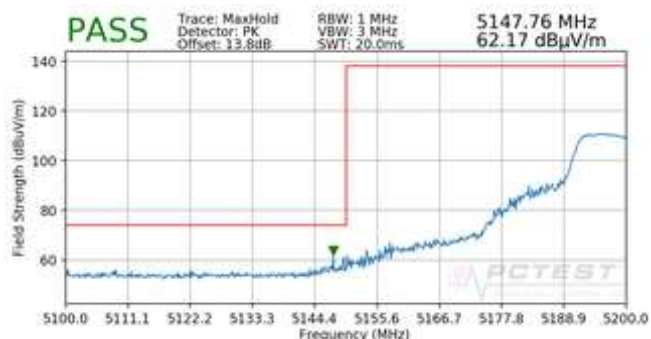
Plot 7-10. Radiated Lower Band Edge Plot (Peak – UNII Band 1)
