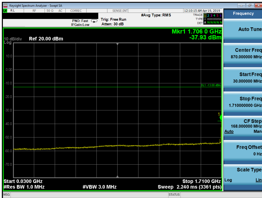
Plot 7-127. Conducted Spurious Plot (Band 66/4 - 20MHz QPSK - RB Size 1, RB Offset 0 - Mid Channel)
