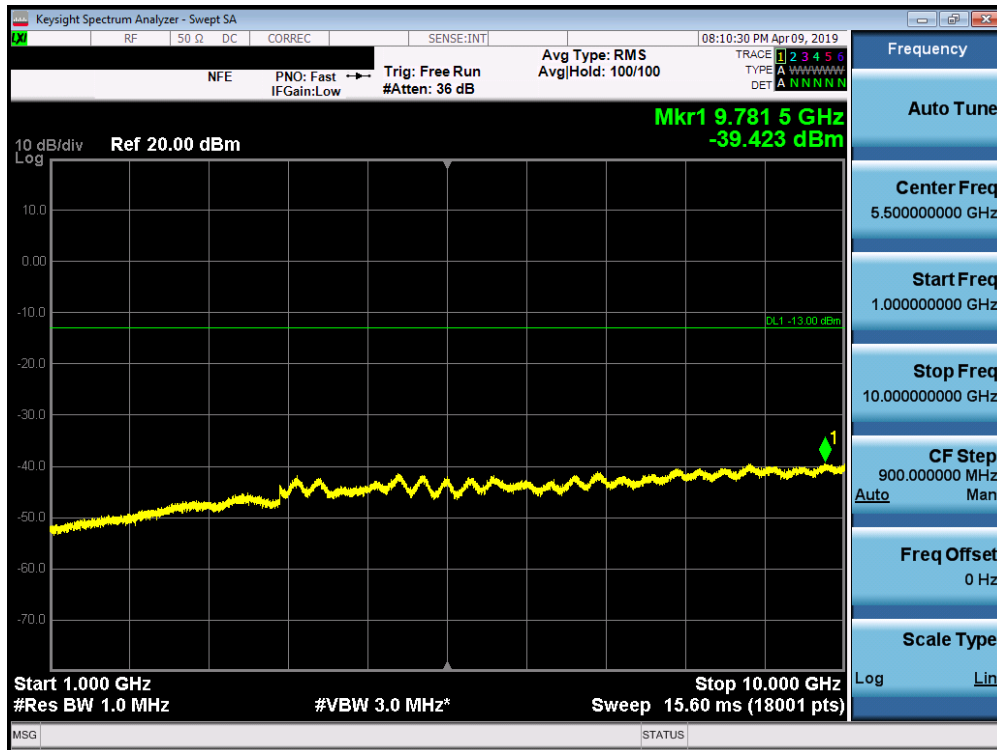
Plot 7-96. Conducted Spurious Plot (Band 71 - 20.0MHz QPSK - RB Size 1, RB Offset 0 - Low Channel)
