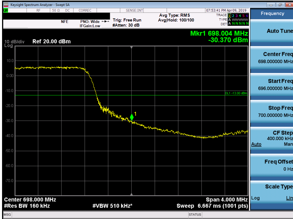
Plot 7-157. Upper Band Edge Plot (Band 71 - 15.0MHz QPSK - Full RB Configuration)
