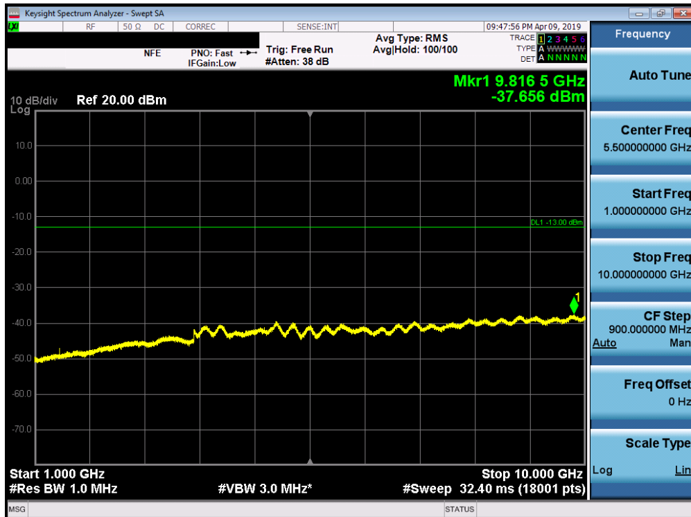
Plot 7-108. Conducted Spurious Plot (Band 12/17 - 10.0MHz QPSK - RB Size 1, RB Offset 0 - Mid Channel)
