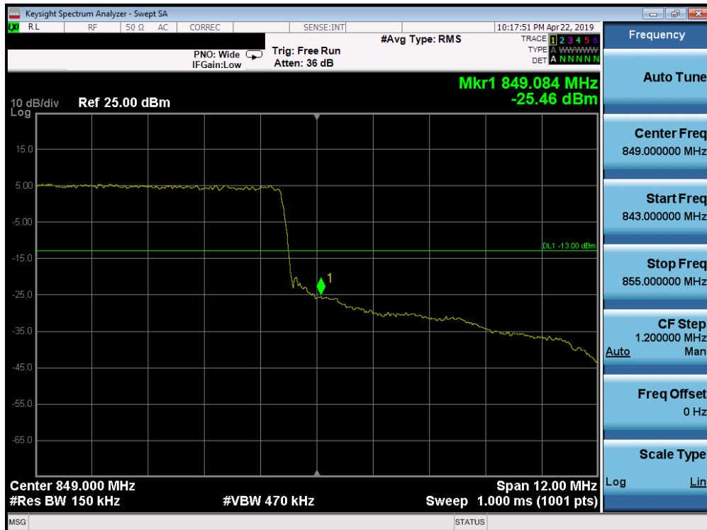
Plot 7-190. Upper Band Edge Plot (Band 26 - 15.0MHz QPSK - Full RB Configuration)
