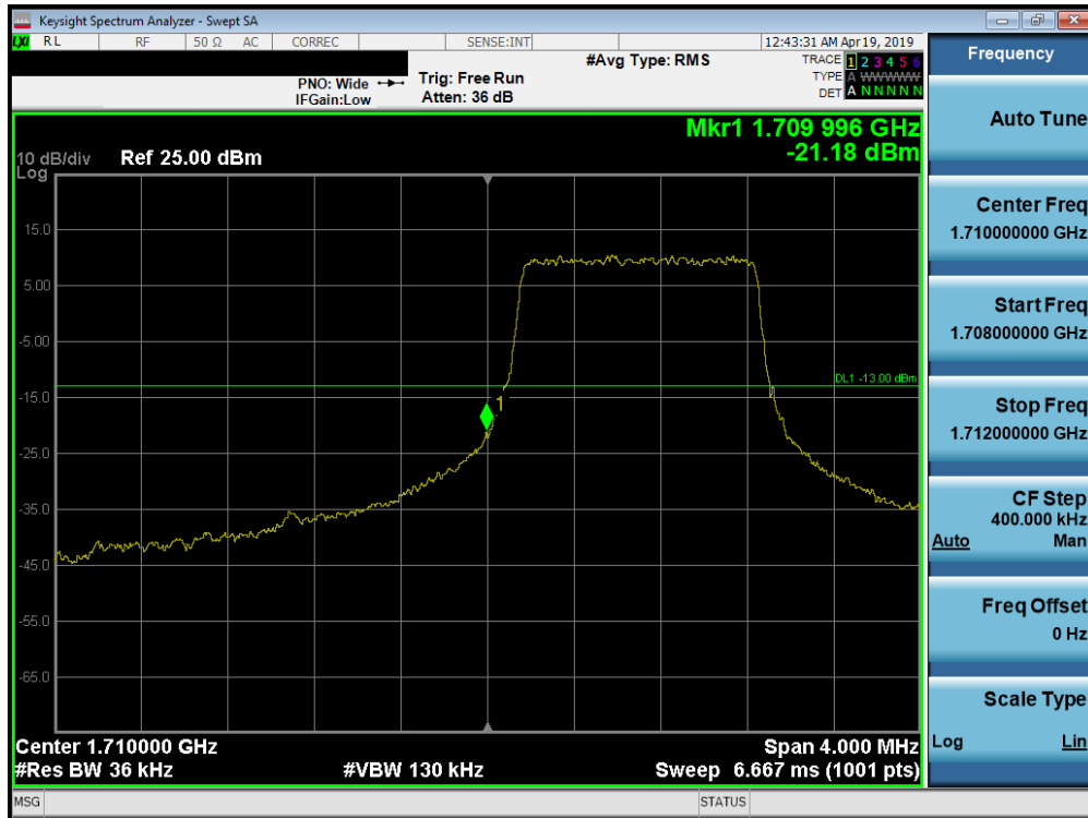
Plot 7-191. Lower Band Edge Plot (Band 66/4 - 1.4MHz QPSK - Full RB Configuration)
