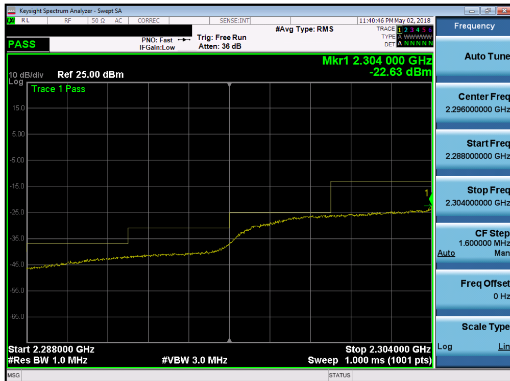
Plot 7-201. Lower Extended Band Edge Plot (Band 30 - 10.0MHz QPSK - Full RB Configuration)
