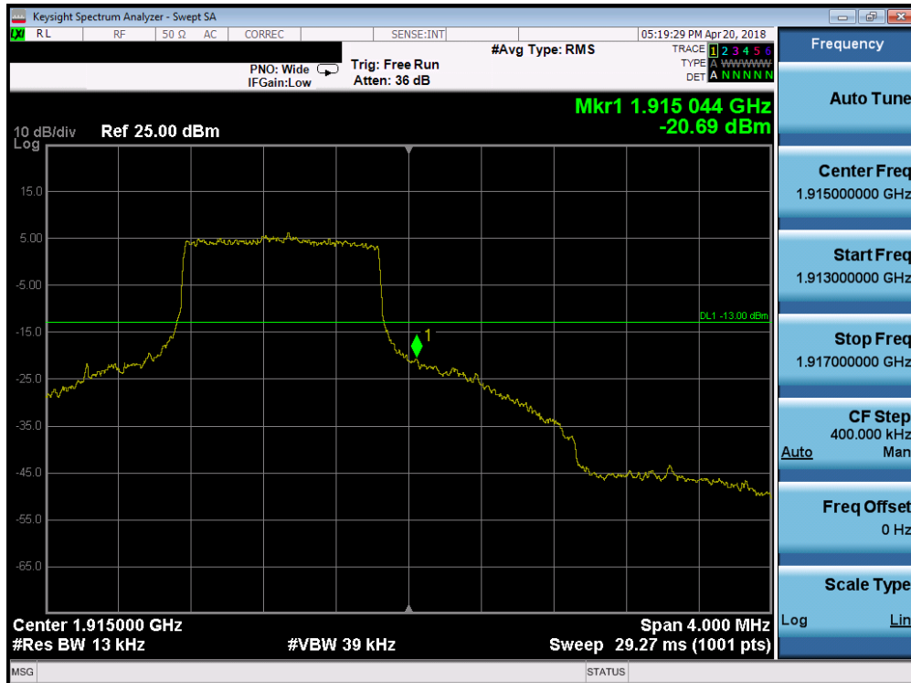
Plot 7-173. Upper Band Edge Plot (Band 25 - 1.4MHz QPSK - Full RB Configuration)
