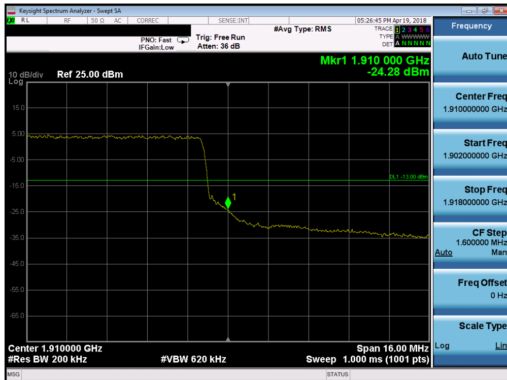
Plot 7-194. Upper Band Edge Plot (Band 2 - 20.0MHz QPSK - Full RB Configuration)
