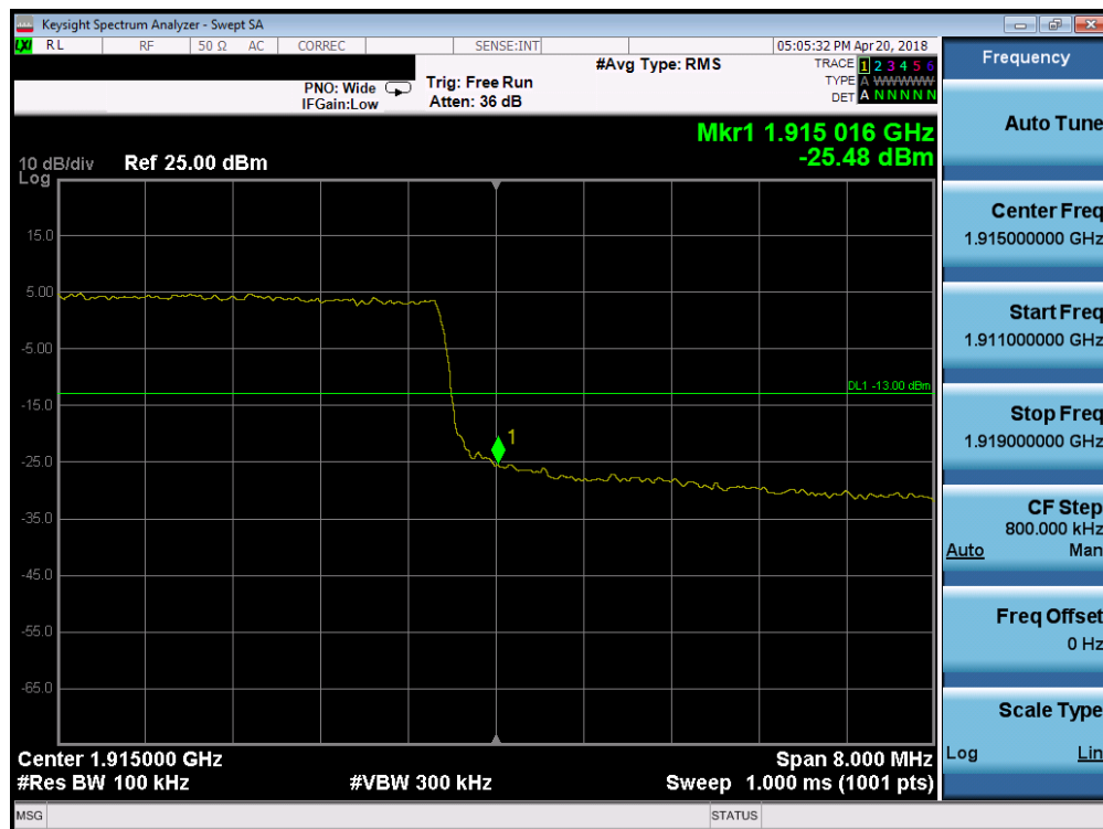
Plot 7-189. Upper Band Edge Plot (Band 25 - 10.0MHz QPSK - Full RB Configuration)
