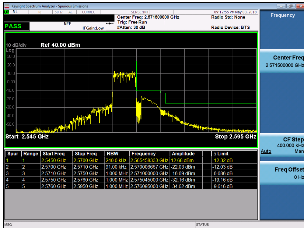
Plot 7-205. Upper ACP Plot (Band 7 - 5.0MHz QPSK - Full RB Configuration)
