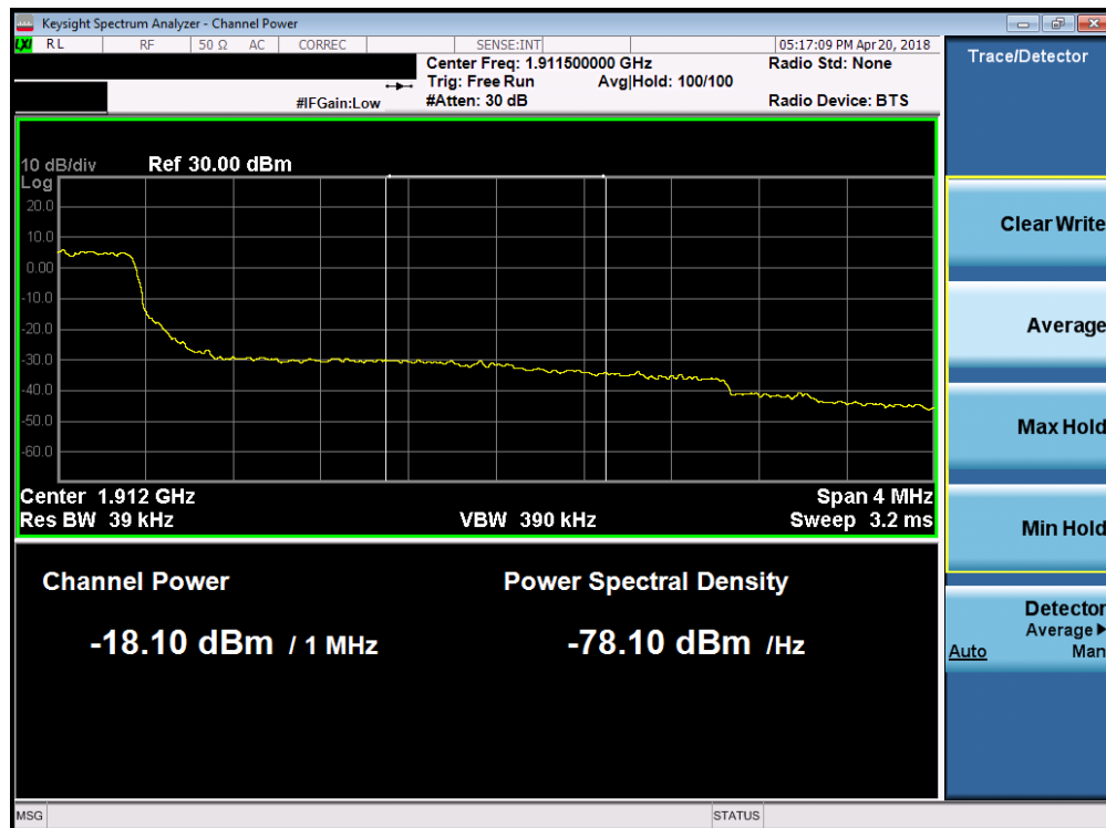
Plot 7-178. Upper Extended Band Edge Plot (Band 2 - 3.0MHz QPSK - Full RB Configuration)
