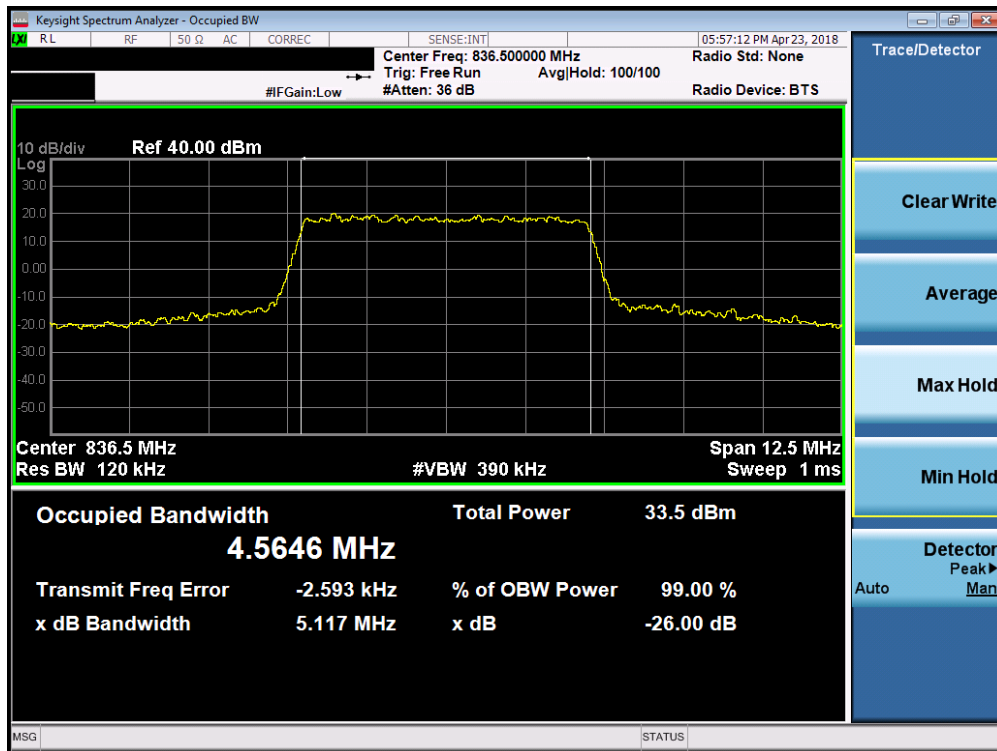
Plot 7-17. Occupied Bandwidth Plot (Band 5 – 5.0MHz QPSK - Full RB Configuration)
