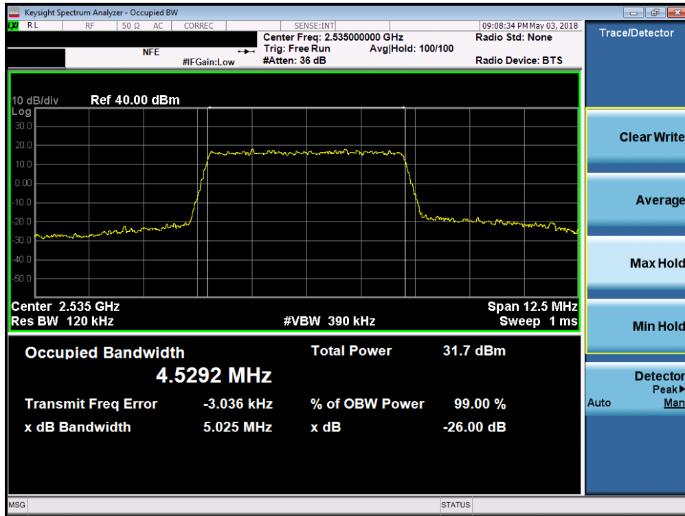
Plot 7-49. Occupied Bandwidth Plot (Band 7 - 5.0MHz QPSK - Full RB Configuration)
