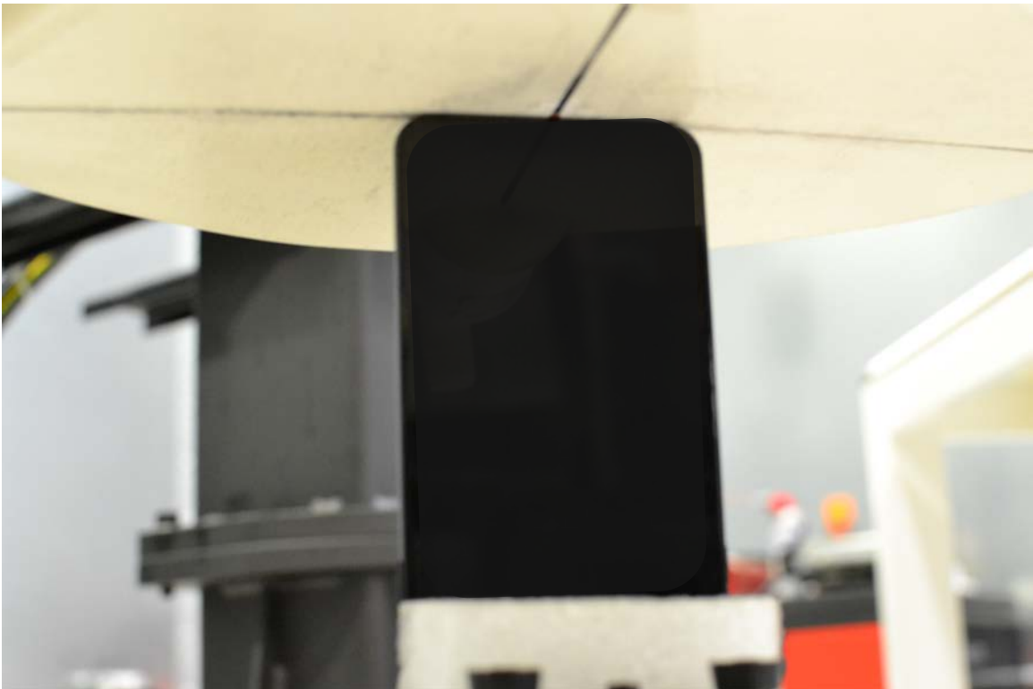
SAR Test Setup Photo 14 – Bottom Edge 0 mm
