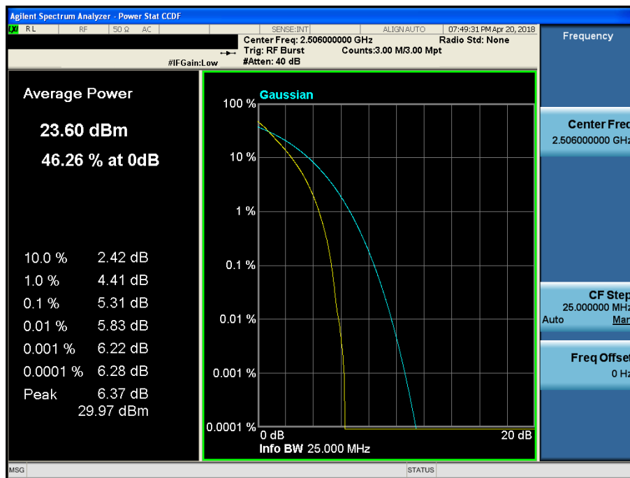
LTE Band 41 / 20 MHz / QPSK - RB Size 100
