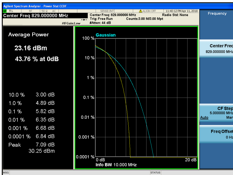
LTE Band 5 / 10 MHz / 16QAM - RB Size 50
