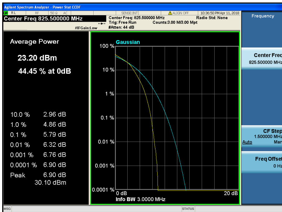
LTE Band 5 / 3 MHz / 16QAM - RB Size 15
