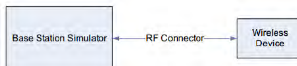
Figure 10.1 Power Measurement Setup
